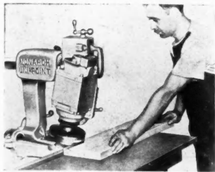
ROUTING is one of the many operations performed by this new lightweight saw.
