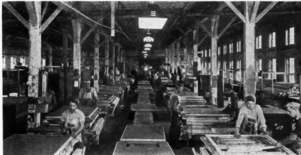
STOUT HOUSES, Inc., have work tables located on both sides of assembly line conveyor.
