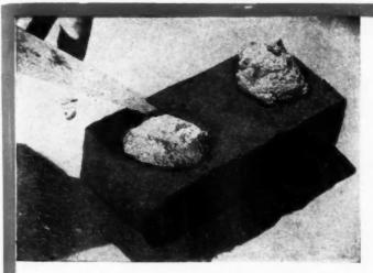
Here's the way to test for high water-retention. Slap a small dab of any two mortars onto a brick. Wait a minute, then feel each dab. The
