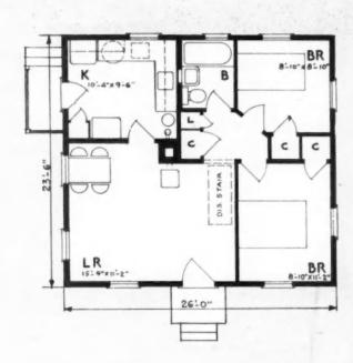
THE PLAN at left provides for basement and attic. The other is basementless with utility room for laundry and heating equipment.
