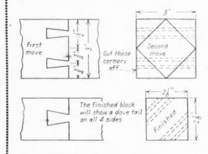
L. H. DUNSON, La Rue, Ohio, submits this idea of a trick splice, not for the added strength that it might inject into the member, but rather because of the improved appearance that it may give to the repair of a table leg or some other piece of furniture. When completed it provides a section of the dovetail on each side of leg.
