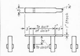
RICHARD H. BARNER, Colwyn, Pa., says: "Here is a jig that I find is much better than trying to use a carpenter's 12" combination try square. It can be moved along the side of the joist and is always close at hand, eliminating the possibility of having it fall into the basement or the first floor as the case may be, which so often happens with the try square."
