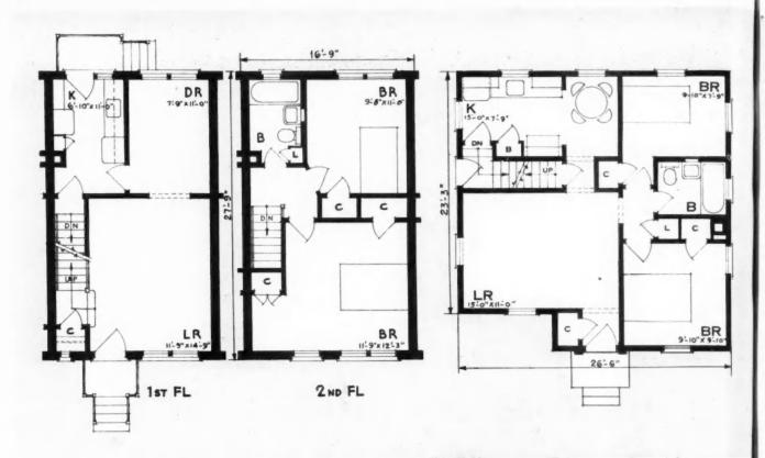
THESE HOUSES—the two-story row (left) and the one-story detached (right)—locate laundry and heating equipment in basement.
