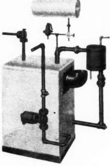
B&G Mydro-Flo Heat is a forced hot water system. The basic operating units are a B&G Booster Pump, B&G Flo-Control Valve, B&G Water Heater and the necessary electrical controls. All are simple, dependable units which can be installed on any hot water heating boiler.
