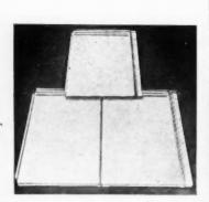
The interlocking side lap aluminum shingle shown above is being applied in photo at left. Head lap of this shingle has two waterbreaks and a vertical safety flange. Completed job with all accessories produces 100 per cent blind nailing for entire roof. Photo: Southern States Iron Roofing Co.
