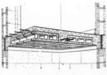
Concrete block joist floor
