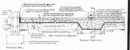
Construction details of concrete floor on ground showing the use of membrane dampproofing.
