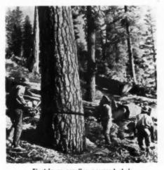
Electric, or gasoline powered chain saws speed tree-falling operations.
