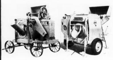
Visual evidence of transformation of Rex concrete mixers to 1946 simplified and streamlined, rubber-tired precision machine.
