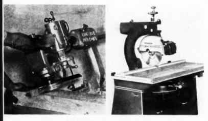
Two Monarch radial saws. At right, heavy duty stationary bench type. Left, lightweight unit that can be carried by two men.
