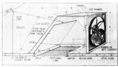
Illustration showing typical attic ventilating fan installation. Drawing: Shreveport Engineering Co.
