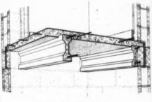
Precast joist floor.
