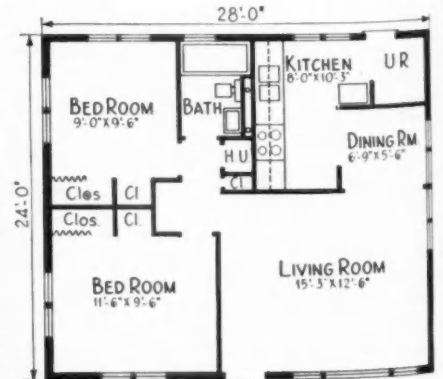
FLOOR PLAN FLOOR plan of five-room Cemesto prefabricated house used by Burns in large project.
