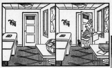
In this utility room there's only one possible place for a modern cabinet-type ironing board — next to the door. The conventional cabinet board would be impractical; would block the entrance, could be used from only one side.
