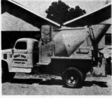
AB2899—Blaw-Knox Co., Pittsburgh, Pa., announce start of regular production on the "Hi-Boy Truk-mixer", the firm's first truck mixer of high-discharge type and its first new design since before the war. The company will also continue manufacture of its horizontal model, which is known as the "Lo-Boy". Unique feature of the new machine is a revolving hopper for both charging and discharging, leaving a gadget-free rear end.
