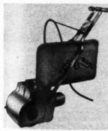
AB2817—The Reid-Way "8" Floor Sander, manufactured by Reid-Way, Inc. of Cedar Rapids, Iowa, makes use of an edger unnecessary in finishing floors. The sander works up to within one-half inch of the baseboard on both sides. The surface speed is 3,534 feet per minute and drum speed is 1,800 r.p.m. It weighs around 85 pounds.
