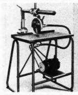
AB2853—Important design changes in the Flexsaw general purpose radial saw are announced by the Flexsaw Co. of Port Austin, Mich. Hand tightening levers have been added, so all adjustments can be made without tools. New precision-calibrated brass plates have been added at all adjusting points to increase accuracy and ease of setting.
