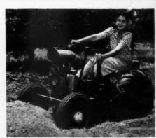
AB2894-The Lincoln Tractor Co., Arcadia, Calif., nces development of a small tractor weighing only 750 pounds, powered by a 6 H.P. motor manufactured by Salsbury Motors, Inc., Pomona, Calif. The tractor has an all-steel welded frame, pivoted front axle suspension, individual rear wheel brakes to facilitate turning and a transmission, providing three forward speeds and two power take-offs for operating mixers, pumps, generators, and saws. Cal des bili
