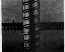
AB28138—The improved design of Hi-Bond reinforcing bars affords greater grip between steel and concrete, eliminating wide cracks, and often makes the use of hooks unnecessary. The interlocking of ribs and firm anchorage of the wires which are easily and quickly affached holds the bars securely in position. Product of Joseph T. Ryerson & Son, they help produce sound structures and lower construction costs through materials and labor saving.
