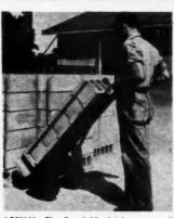
AB28161—The Reed Block-Man, a product of the R. S. Reed Corp., Three Rivers, Mich., is a hand truck with forks which enables one man to pick up and transport six concrete blocks at one time. The bottom block on each pile is laid face down and thereafter serves as a pallet. The loaded truck will roll freely over soft ground.
