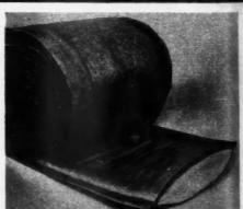
AB28133—To meet the demand for completely enclosed, envelope-type insulation, The Gilman Brothers Co., Gilman, Conn., has developed a new type Cellulite—flame-proof cotton building insulation. The new Type E Cellulite has a sturdy vapor seal on one side and a tough paper covering on the other. It is made in the same standard widths as the regular Cellulite and is packaged in certons for easy shipping, storage and handling.
