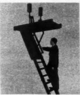
AB28225—A new line of folding stairways that disappear into the attic, requiring no springs and no floor space to operate, is now available from Precision Parts Corp., Nashville, Tenn. Made of kiln-dried poplar with brackets and rocker arms of cast aluminum and hinges of cast brass, they are actuated by simple counterweights.
