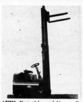
AB2824—New style uprights on the Clark Tructractor Clipper truck permit higher tiering with this model, the 2,000-pound capacity unit. Overall height of the basic standard lift is 83 inches with forks lowered and permits passage through 7 foot doors. Maximum tiering height has been increased from former 108 inches to 124 inches.
