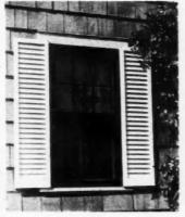
A82872—Leigh ornamental metal shutters, shown above, are manufactured by Air Control Products, Inc., of Coopersville, Mich. Available in a wide range of sizes in louver or panel design to fit any standard window. Made of heavy gauge metal of welded construction. Shutter held in place by four screws or nails for quick installation.
