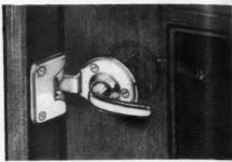
The IVES Non-Mortise Latch is as easy to install as a rim latch - as neat as a mortise lock. It is made in brass or steel and is now available for prompt delivery. It is unsurpassed for easy latching and features attractive cast handles . . . longer spindle which adjusts automatically for %" to 1 %" doors and can be adjusted to 1%" . . . improved strike allows for sagging of door.
