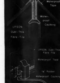
Application Direct to Studs. Provide continuous nailing base for all edges. Nail Upson Floating Fasteners to studs on 16" centers. Apply by first clinching Fasteners in center of panel, Leave 16" space between butt ends of panels. Nail edges of panels every 16". Use Upson Waterproof Tape on panel edges around built-in bath tubs. Enamel entire surface of panels before applying mouldings.
