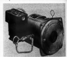
AB2878—A revolutionary, horizontal-vaporizing type oil burner known as "Conco-Breeze" is being made by Conco Engineering Works, Mendota, III. Since gassification is complete within the burner proper, refractory linings and refractory combustion chembers are not essential. The unit is complete with controls for fully automatic operation on warm air furnaces, steam and hot water boilers, domestic hot water heaters and coal-burning space heaters.
