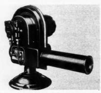
AB28195—The new Norge Heat oil burner, Model COB-13 is a ½-gallon-capacity gun-type unit which utilizes the basic principles of controlled combustion found in the Whirlator Head of the Norge Heat winter air conditioners. Primary air and secondary air mixing with fuel is constantly controlled, with special dials on the outside of the burner for ready adjustment. Model COB-13 will burn straight distillate, catalytic stock or No. 1, 2 or 3 fuel oil.
