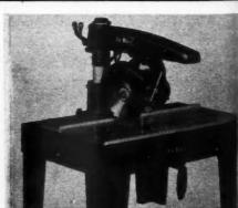
A828120—DeWalt, Inc., Lancaster, Pa., have released a new Cut-Master model. Combining the functions of many machines, this machine is designed for all-purpose cutting. Simple mechanism alignment adjustments are provided to maintain the accuracy of every setting. A new kick-back device is an exclusive safety feature for ripping. A wide work-table provides ample space for the handling of materials or for gang cutting jobs. Paul, porch is in in bac
