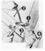
rial. Devised by the C. B. Tool Co., Lancaster, Pa., for use on rough, warped, or twisted lumber, it requires only four simple manipulations to operate: (1) Start nail in board as usual; (2) With stroke of hammer set anchor pin; (3) Draw handle down until groove is closed, and (4) Hold, drive your nail.
