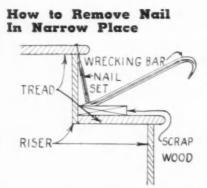
**T**HIS suggestion is made by Alex Iseppon, 484 Portage Road, Stamford Centre, Ontario, Canada. For example, to remove a nail that has come through the good side of a stair riser, put a scrap piece of board on the tread below the nail; put a nail set on the point of the nail, then put a pinch bar under the nail set and on top of the scrap piece of wood. Push down on the pinch bar to force the nail up. American Builder, April 1948.
