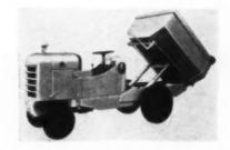
Its overall height is only 5 feet, 8 inches. The dump body is ideal for trucking sand, slag, castings, coal, cinders, gravel, ore, concrete or other bulk material. Built as a companion to the Payloader Shovel, the Payloader Buggy matches it in capacity, compact size, speeds and operation. In addition, all main parts of the Buggy are interchangeable with those of the Shovel.
