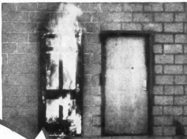
Picture shows absolute protection afforded by Weldwood Fireproof Door. After withstanding an intense fire for sixty minutes, the Weldwood Fireproof Door still prevented passage of fire, smoke, heat, gases and remained cool to the touch on the unexposed side.
