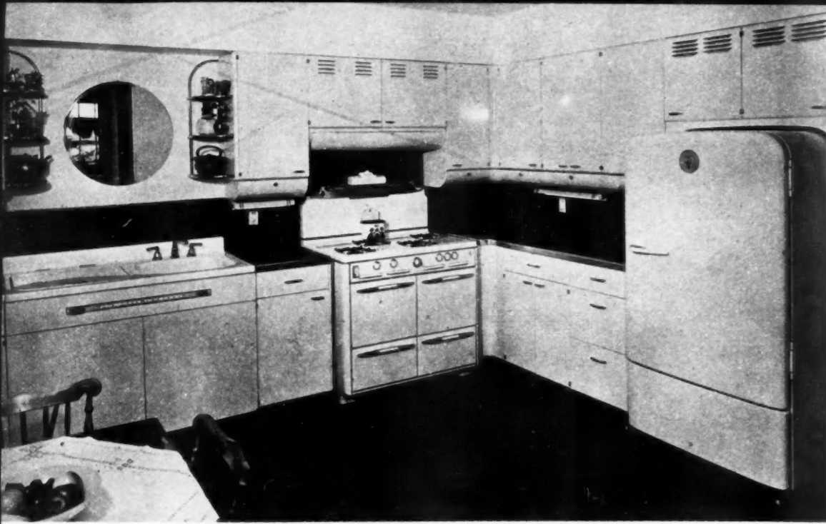
THIS kitchen was planned in accordance with new principles developed in an extensive research study conducted by one manufacturer. Note that range is between the sink and refrigerator
