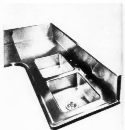
IN THIS stainless steel sink, product of Just Manufacturing Co., the sink bowls are welded electrically to drainboards to eliminate seams or soldered joints. Heavy gauge material is reinforced by under-structural channels. The manufacturer will fabricate sink and drainboard units to any special size or shape builders may require
