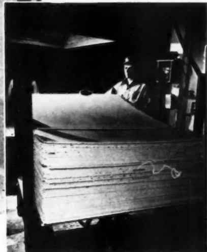
AT LEFT the Prespine panels are emerging from the huge press which forms them by extreme pressure and heat. Above, the freshly pressed board is being loaded on a truck and transported to trimming and sanding machinery in main plant
