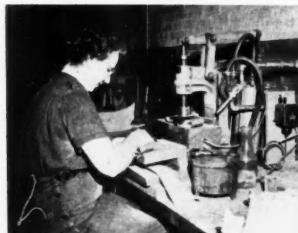
ABRASIVE BELTS for sanders are cut in lengths on pneumatic-operated machine developed by factory. Belting is bought in mile lengths by power tool producers
