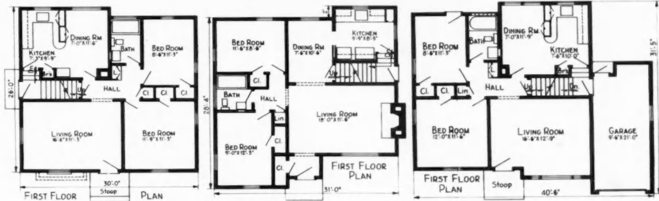
THESE floor plans are typical of those used throughout this 250-house development. Prices vary from $10,450 to $14,500
