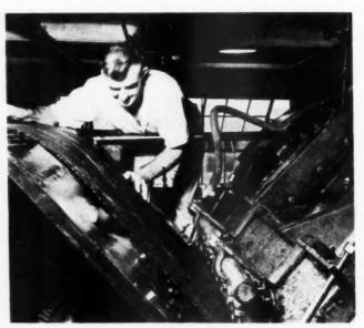
HERE the material is carefully fed into a punch press where it is die-cut into tile with square edges
