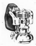
of jobs. It will not stall under any service requirements. It operates on 115 volts, 25 to 60 cycles, A.C. or D.C. The disc is precision balanced, 7 inches in diameter, with a reinforced pad, fabricated from heat and oil-resistant rubber, bonded to it. Sandpaper is attached by a positive nut clamp. Speed of the disc is 3,000
