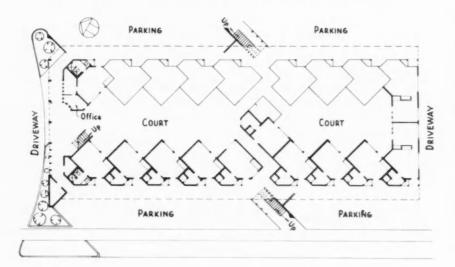
BECAUSE of space limitations, it was not possible for Architect Burton A. Schutt to design a conventional motel on the site chosen for this structure. With the lot only 100x200 feet, it was necessary to incorporate motel-type units in a hotel design. Intended to provide middle-class accommodations for motorists traveling Wilshire Boulevard in Los Angeles, the pleasing combination achieved here has permitted the motel to enjoy the income of a luxury hotel.
