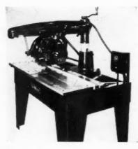
Model GR is actually a complete saw shop in one machine, according to its manufacturers. It is a cut-off saw, a miter saw, a rip saw, a tilting arbor saw, a double miter saw, and a variety saw. Using the proper cutting tool, it's a dado machine, a gaining machine, a grooving machine, a rabbeting machine, and a shaper. The machine is adapted to these various operations by simply changing the cutting tool.
