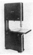
jobs but for home work shop users is on the market. All castings are heat treated before machining to relieve stress and distortion. The heavily-ribbed, 14 inch by 14 inch, table surface is ground smooth and tilts a full 45 degrees right and 15 degrees left angle. The wheels have Neo-prene tires for oil resistance and wearing features. Each wheel is balanced for smooth and quiet operation. This band saw is the newest addition to the line of wood-
