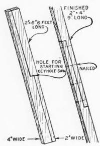
mark off the 2x6 as shown in the sketch and then rip along the mark from both sides. Where these slits meet at the exact center, I drill a hole for starting the keyhole saw. I then cut away the remaining two inches of the mark. The final step is to spike the two pieces together with long nails. A 2x6 four feet long will make a 2x4 six feet long; a six-foot piece will make a nine foot 2x4; a ten foot piece will make a 2x4 fifteen feet long, and so forth.
