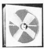
is easily installed in the window, or in the attic. In addition, its capacity, rated at approximately 7,000 C.F.M., makes it equally applicable to business and industrial establishments. Powered by a 1/4 H.P. motor, this air mover operates quietly and economically. Its overall dimensions are 36 inches by 36 inches, and it is furnished with an attractive grille.
