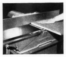
head can be adjusted tangent with the cutting circle on the knives. When not in use, the equalizer bar can be hinged back in the rabbet ledge, slightly below the surface of the rear table. To plane wide stock, the bar is folded back out of the way and the
