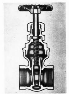
CROSS section of gate valve showing unrestricted flow channel
