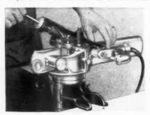
SHARPENS ITS OWN CUTTER—Just set it up in the Bench Bracket and use the simple Grinding Attachment.
