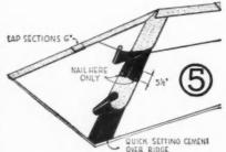
Bend these strips lengthwise through the center and "shingle" them on the hip or ridge. Start at the lower end of the hip or at either end of the ridge and lap each strip 6 inches over the lap end of the preceding one.
