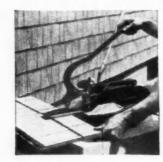
A new Grip Cutter, now offered by La Belle Industries, Inc., Oconomowoc, Wis., is adjustable to handle all types of insulating siding up to one inch thick.
