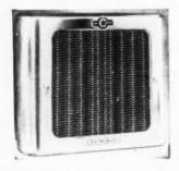
Electromode Corp., Rochester, N.Y. Known as the Bilt-in-Wall Small-Room Heater, it is easily installed in practically any type of wall construction. The heater connects to the regular 110-volt A.C. house circuit. It is rated as 1,320 watts. A quiet built-in fan distributes 80 cubic feet of heated air per minute. Heat is generated by a patented cast aluminum heating element which has no exposed wires or coils. The heater is equipped with a thermal safety switch that prevents overheating.
