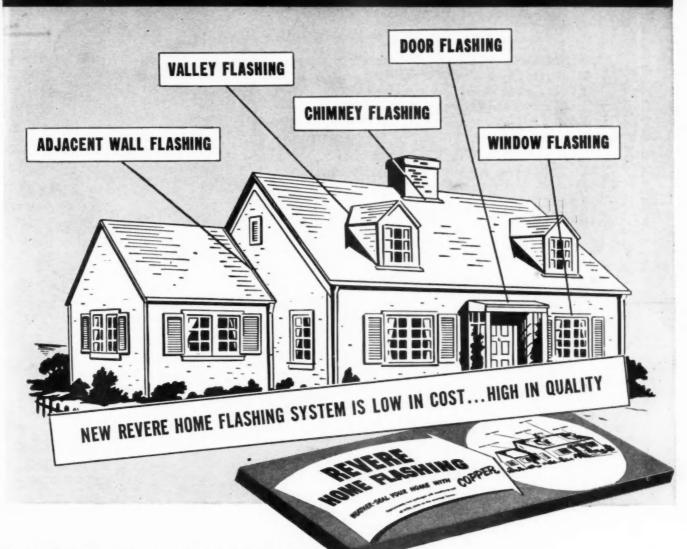
IT'S so low in cost . . . so economical to install, that Revere Home Flashing enables even low-cost houses to have the lasting protection of durable, non-rusting copper flashing!
