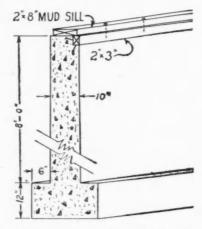
necessary to bore holes for bolts. Just spike the mud sill to the 2x3. Submitted by J. JEROLD NORMAN, Oswego, Ore.
