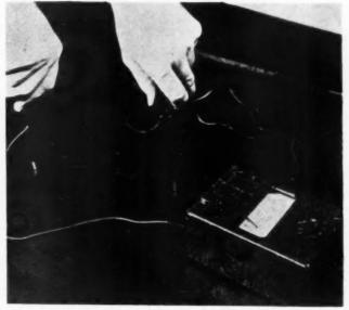
**9.** TESTING an asphalt tile floor for conductive resistance. Asphalt tile far exceeds the safety margins
