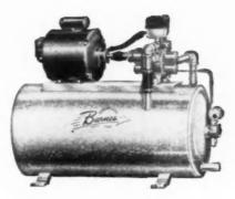
with a 1/4 or 1/3 H.P. electric motor. It delivers up to 420 G.P.H. at 30 pounds discharge pressure, with suction lifts up to 22 feet. Maximum pumping pressure is 40 pounds for the 1/4 H.P. system, and 60 pounds for the 1/3 H.P. system. The water system requires no plunger, rods, packing glands or drive pulleys for operation. Two helical impellers, turning at motor speed (1750 r.p.h.), give an uninterrupted, non-pulsating flow of water.
