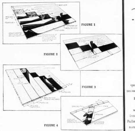
NINETEEN-INCH selvage, doublecoverage asphalt roll-roofing is produced uniformly as a 36-inch wide sheet, 17 inches of which is mineral surfaced, and 19 inches unsurfaced. The 19-inch selvage, or unsurfaced, portion is finished in various ways by different manufacturers. Some manufacturers saturate the sheet and others modify it in other minor ways.
