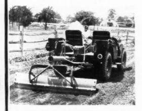
Howard Schneider, Shrewsbury's partner, says, "Our 'Jeep' is never idle. We use it for digging, grading and cleaning up after jobs, as well as a pick-up and tow truck. We often carry loads of 1200 lbs. or pull trailers of 2 1/2 tons."
