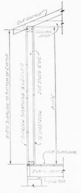
Gyprock sheathing on the outside and Sheetrock on the inside of the wall.
