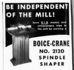
You can turn out commercial grade sash, fine mouldings, coped joints, stair treads, drawer and cupboard fronts and do other millwork yourself.
