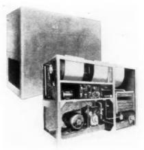
circulates and ventilates air for ideal working and living conditions. Available in nine sizes, ranging in capacities from 3 to 40 tons, a single threein-one unit houses the refrigeration compressor section; the air cooling, dehumidifying and circulating section; and the evaporative condenser section.
