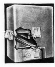
tion to the furnace is necessary that day or night, since it is regulated through draft dampers automatically operated by a thermostat. Three operations are required when tending the furnace, and these may be completed in about two or three minutes. In this heating plant, soft high volatile coal is turned into coke by transforming coal into gas and burning it as it comes from the coal.
