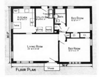
masonry placed on poured concrete trench walls 4 feet deep. A four-inch thick concrete mat is placed over the entire floor area. The mat is laid over a bed of cinders between vapor barriers. Asphalt tile cemented to concrete slab is used in all rooms. Steel casement sash are used in all window openings. Asphalt shingles cover the roof. For the interior all walls and ceilings are plastered,
