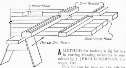
This jig can be used on the job for cutting studs, blocks, and bridging, with a portable power saw. It is not as flexible as a radial arm saw, but more economical.
