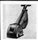
AB2707 — American Rental floor sander. American Floor Surfacing Machine Co., To-ledo, Ohio. Working parts in two units for quick replacement. Motor, vacuum fan with drive pulley in one unit, with 8-inch sanding drum, shaft, bearings in other.
