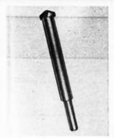
A829368 — Masonry drills. Kennametal, Inc., Latrobe, Pa. His high carbon steel shanks and a cutting blade of solid Kennametal. Blade has high resistance to wear and shock. Bit is used to drill file, slate, stone, marble, brick, cement, plaster, asphalt, porcelain, micarta, and other nonmetallic materials.
