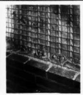
AB27197—Steeltex for brick or stone veneer. Pittsburgh Steel Products, Pittsburgh, Pa. The brick or stone is built into and thoroughly bonded to a 1-inch slab of cement mortar which is reinforced with a network of heavily galvanized copper-bearing steel wires. Produces solid wall without other sheathing.
