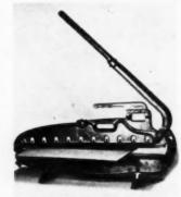
AB29154—Asbestos Siding and Shingle Cutter. Tri-States Building Materials Co., Ft. Worth, Texas. Equipped with two high-grade steel cutting blades 32 inches long. Has bolt adjustment for adjusting upper and lower blades. Cuts any thickness of asbestos siding or shingles. Weighs 37½ pounds; is 36½ inches long.
