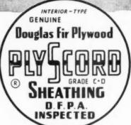
PLYSCORD — identified by this "grade-trade-mark"—is the sheathing grade of Interior-type Douglas fir plywood, manufactured in strict accordance with U. S. Commercial Standard CS45-48. It has a face panel of C veneer and a back panel of D veneer. Plys are bonded with highly water-resistant (but not waterproof) glues; the material will withstand occasional wetting such as might ordinarily be encountered during construction.
