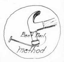
Greater strength is obtained through toe nailing when a slight crook is made at the point of the nail.
