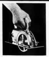
AB29199—Guild Saw, Model A-4. The Porter-Cable Machine Co., Syracuse, N.Y. This 4½-inch saw can be tilted for bevel or compound mitre cut. Has adjustable ripping guide. Uses include dadoing, cutting tenons, grooving and notching. Can be used for cutting overhang of house siding, roofing, floors; for cabinet work.
