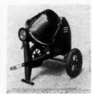
AB2970—Wonder "3" trailer mixer. Construction Machinery Co., Waterloo, Iowa. Half-bag capacity of any mix up to 1:21/2:4. Electric welded frame, cantilever springs, pneumatic tires for high speed trailing. Engine, 11/2 H.P., air-cooled, housed.
