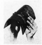
AB29205—A flooring material named Terraflex. Johns-Manville Co., New York, N.Y. Is extremely flexible. Slightly heated, it can be curved to form stair nosings and coved bases. This quality permits floor to conform to any uneven surfaces and provides unusual resilience and comfort under foot. Offered in varied colors.
