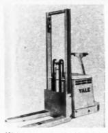
AB29169—Low-cost high-lift Work-saver electric pallet truck. The Yale & Towne Mfg. Co., Philadelphia, Pa. Has 2,500 pound capacity. Is bettery-operated both for travel and lifting loads. Is 39 by 31 inches in overall dimensions. Lifts pallets & inches for overhead tiering. Available for immediate delivery.
