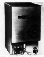
AB29194—Oil-fired floor furnace for low-cost housing. Northwest Metal Products, Inc., Seattle, Wash. Model FL-200. Output is 50,000 B.T.U. Features include electric draft booster fan as standard equipment, small register grill, easily removable burner pot. It is available with both manual and automatic controls.
