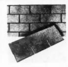
AB29268—Gient strip asphalt shingles. Johns-Manville, New York, N. Y. Felt base saturated and coated with refined asphalts. Granules imbedded in coating mineral, then second coat of asphalt and second coat of mineral granules are added next.
