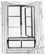
AB29115—Bedroom window with hopper ventilator at sill. Detroit Steel Products Co., Detroit, Mich. Protects from drafts by deflecting air toward ceiling through use of intilting sill vent. Frames and sash are of steel. Cam action lock draws vent tight shut. Precision fitted at factory. Has complete safety features.
