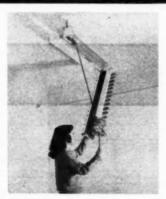
AB29218—Fluorescent fixture called "Guth-Lite." The Edwin F. Guth Co., St. Louis 3, Mo. Equipped with "Jacknife" hinge which permits maintenance from floor. A maintenance rod releases latch which permits entire assembly to swing down on Jacknife hinge. Entire assembly can then be cleaned and repaired.
