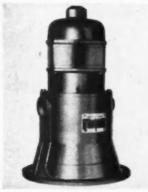
AB29136 — Self-priming centrifugal pump. Marlow Pumps, Ridgewood, N. J. The 10EV series have but one moving part. With 35 foot total head will deliver 34 gpm with ½-horsepower motor. Made in three sizes—½, ½, and ½ HP. Does a score of pumping jobs with minimum of attention. Positively self-cleaning.
