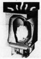
AB29376 — Automatic thermostatic control oil-burning floor furnace. H. C. Little Burner Co., Inc., San Rafael, Calif. For moderately-priced homes. Features 3 volt electric hot wire ignition. A catalytic oil heat control allows operation on No. 3 furnace oil. Thermo limit control prevents overheating of floor grille.
