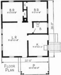
model summer cottage. The interior is partitioned off into four rooms with plasterboard on one side leaving the other side to be finished later. The cottage has no ceiling. This also can be done at some later date.
