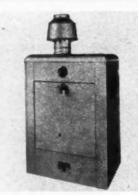
AB29189—Gas-fired hot water boiler for small dwellings. A. O. Smith Corp., Milwaukee, Wis. Will operate on any type of natural, manufactured or liquefied gases. Is 3 feet high, 2 feet wide, and 18 inches deep. Especially suitable for radiant heating, it operates equally well with other systems.
