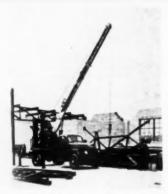
AB2997 — Hydrocrane. Bucyrus-Erie Co., South Milwaukee, Wis. Model H-3, 3 ton, ½-yard is fully hydraulic in operation. Boom telescopes and hoists hydraulically; load hoists hydraulically; deck revolves hydraulically; outriggers are set hydrauliclly; bucket digs hydraulically. Safe system. Simple to maintain and operate.
