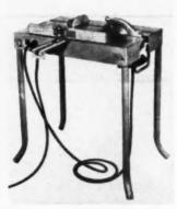
AB29374—Saw table. J-P Manufacturing Corp., Selinsgrove, Pa. Designed for use with a Skilsaw. Table top is of ½-inch steel, one piece construction. Overall, 26x17 inches with sides 4 inches high. Skilsaw is fastened with 4 clamps. Mounted it becomes table saw and electric hand saw. Designed to prevent tipping.
