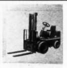
A82965 — Yardlift-40. Clark Equipment Co., Battle Creek, Mich. Wide drive axle, dual tires. For high lifts more than 144 inches. Easily attachable fenders included. Smooth operation over soft ground and surfaces unsafe for solid tired machines. Easy to use.
