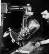
Straight ripping or bevel ripping is easy with Radial SKIL Saw. The operator simply slides the material along the riptence for accurate cuts.
