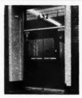
AB29133—Glass door frame. Pittsburgh Plate Glass Co., Pittsburgh, Pa. For use with Herculite tempered all-glass doors. Heavy, anodized and extruded aluminum reinforced with steel channels and tierods. First of its type, Available in 12 standard patterns. Includes checking floor hinge, top pivot.
