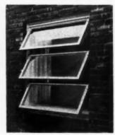
A827206 — Wood awning windows. Gate City Sash & Door Co., Fort Lauderdale, Fla. Windows are furnished complete with hardware and glass already installed, and screens semi-prefit and wired with Lumite. Wood stool and apron included. Vertical weather stripping included. Sash operates smoothly by a crank.
