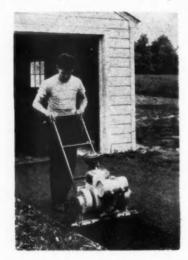
to curbs, rails, manholes, buildings or fences. Requires no water. Impactor plate heated by engine exhaust. Travels under its own power when working. Powered by its own power when working. Powered by 21/2-H.P. Wisconsin Model AB air cooled engine. Working speed on level ground is 35 to 42 F.P.M., depending on type of material and thickness of mat. Wayer material and thickness of mat. W Impactor, Inc., 12. North Third Impactor, Inc., 12 Columbus 15, Ohio. St.
