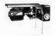
volt, 60 cycle, three phase AC. Motor size furnished depends on door to be handled. A centrifugal clutch allows motor to come up to speed before starting load, and clutch will slip when normal driving load is exceeded by more than a reasonable amount. This affords protection to door, automobile and persons. Handles door sizes up to 400 square feet. Barber-Coleman Co., Rockford, III.
