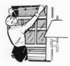
blind stop and drawn taut at sill with thumb screw. Tension is maintained on sides by five strand salvage edge, and "free floating" sill bar at bottom corrects out-ofsquare sills. Keystone Wire Cloth Co., Hanover, Pa.
