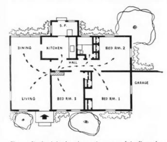
The gas-fired unit is placed near the center of the floor plan, and distributes heat in three directions from registers located 6" below ceiling level. Through the use of the jet principle heat is circulated at a velocity of 300 feet per minute to all parts of the house. Test showed a room-to-room temperature differential of less than 2°.
