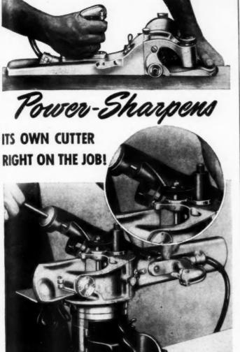
Keep your power plane cutter sharp on the job. You can resharpen the cutter in a matter of minutes, sharp as new. Just set the plane in the bench bracket, remove the cutter arbor and replace it with the grinding arbor and wheel. Mount the grinding attachment on the plane and switch on the power.
