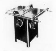
sert provides full support to work. From front edge of table to center of blade, distance is 15% inches. Blade guard rides with work. Can be run by any standard  $\frac{3}{4}$ or  $\frac{1}{2}$ -H.P., three phase, single phase or DC motor, for all common voltages and frequencies. Delta Manufacturing Div., Rockwell Manufacturing Co., American Building, Chicago, III.
