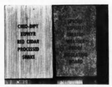
DOUBLE WALL CONSTRUCTION OF CREO-DIPT ZEPHYR SHAKES AND UNDERWALL OF SPECIAL INSULATING BOARD
