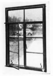
offering smooth base for finishes. Double weathering contact all around frame and ventilator. Corners mitered and butt welded. Sections designed with ample room at jamb for attaching screens and storm windows. The Steelcraft Manufacturing Co., Rossmoyne, Ohio.
