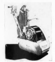
is turned on, it starts under "no-load" condition, due to automatic V-belt take-up. As motor gains speed, pulley squeezes V-belt from side and belt then turns drum. Simple push-button speed control in ranges from 1,600 to 2,800 R.P.M. in 200 R.P.M. gradations. When dial is turned, diameter of drum pulley is changed, varying speed, Easy servicing. Variable drum pressure from 52 to 103 pounds. American Floor Surfacing Machine Co., Toledo, Ohio.
