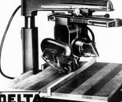
Model 40A, shown, is a cabinet-base machine with a rip capacity up to  $3\frac{1}{4}$ ". Also popular with builders is Delta Multiplex Model 30A with cabinet base and a rip capacity up to  $2\frac{1}{4}$ ". Either machine is easy to take right to the job; two men can carry and load it on your fruck. Both models are widely used for cutting foundation forms, sheathing, roofing, cabinets, doors, frames, drawers, sills, stair treads, etc.
