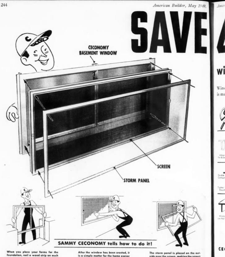
When you place your forms for the foundation, nail a wood strip on each side of your opening to provide vertical rebates. Strip forms, lower attached fins of Ceconomy Basement Window into rebates. Plumb and level. Grout with concrete.
