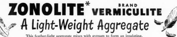
This feather-light aggregate mixes with gypsum to form an insulating, crack-resisting, fire-retarding plaster. Mixes with cement to form a light-weight permanent insulating concrete. As a concrete or plaster, it will never burn, rot or decompose.
