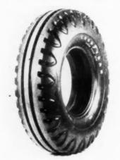
help to eliminate hard steering and vibration in these types of operations. It is known as the Hard Rock Rib. Tread design consists of three heavy circumferential ribs. Goodyear Tire and Rubber Co., Akron, Ohio.
