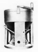
can be operated manually or by compressed air. Operated by air, bucket gates close instantly when supply hose valve is released or when nozzle is pulled from bucket air socket. Six-foot diameter 4-yard size weighs 4,000 pounds. Koehring Co., 3026 W. Concordia Ave., Milwaukee 10, Wis.
