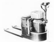
either right or left hand operation, threepoint suspension for smooth travel over uneven surfaces and differential-action trailer wheels that eliminate wheel scuffing. Automatic power cut-off instantly cuts off power supply to motor upon release of control handle, and applies positive quickacting brake to drive shaft, immediately stopping truck. Towmotor Corp., Cleveland 10, Ohio.
