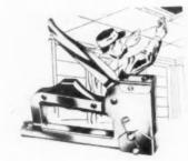
tacker, driving a heavy 1/2-inch staple which toes-in when driven, resulting in strong holding power. Fastener Corp., 860-902 Fletcher St., Chicago 14, III. (Continued to page 164) The jolt rugg nific: And to at smoothis
