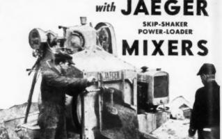
Jaeger 65, 115 and 165 Mixers pour more concrete per day because they have famous "Dual-Mix" drums for faster mixing and discharging charging skips that load while the previous batch mixes then rise and shake their loads into the drums fast and clean, automotive transmissions, big clutches, oversize engines, and fast skip-hoisting and lowering device. They all mean greater production per wage dollar. Write for Catalog M-8.
