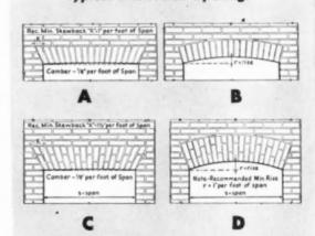
Figures A and B show arches with continuous soldier courses. Figure A is made of brick with tapered sides and ends while Figure B shows brick with tapered sides only. Figures C and D show arches built of soldier and header combinations, staggered in alternate courses, with Figure C made of brick with tapered sides and ends and Figure D of brick with tapered sides only.
