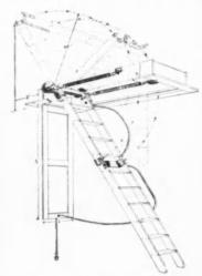
be finished in color desired. Stair hinges at about center, rotates upwardly on shaft fixed into the well. Operates easily. Locked in down position by automatic locking device. Time required to install: about 30 minutes after well is made. about 30 minutes after well is made. Foldaway Stairway Co., Inc., 813 Seaboard St., Portsmouth, Va.
