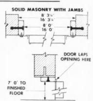
PROPER preparation of the garage door opening for all steel doors is of the first importance if doors are to be installed quickly and easily and operate satisfactorily.
