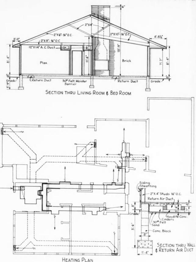
HEATING arrangement is shown on the floor plan above. The grey tone on ducts indicates the supply of warm air in winter and cool air in summer. These ducts extend above the line of closets on both sides of bedroom hall. Dotted lines indicate return ducts under floor. Entire area under concrete slab of equip-
