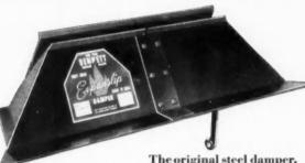
\*Expanslip STEEL DAMPER The original steel damper. Exclusive "Slip-Joint" avoids damage to masonry from heat-expansion. No breakage in shipping, handling, installation or use. It's the only damper with 60° Steep-Slope. High dome insures best results. Lays up with minimum cutting or fitting. Competitively priced. Sizes 24", 30", 36", 42", 48", 60" and 72". Cat. No. C-101.
