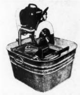
tub which serves for both preliminary soaking of the tile and as a coolant container.
