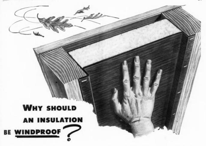
A 15-mile wind penetrates a 13-inch plain brick wall at the rate of 7 cubic feet per square foot per hour. It penetrates a conventional frame wall at .13 cubic feet per square foot per hour. If occupants of the house are to be comfortable, an efficient insulation must guard against such air infiltration.
