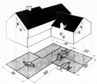
PERSPECTIVE shows ground surface covered by roof Figure 4
