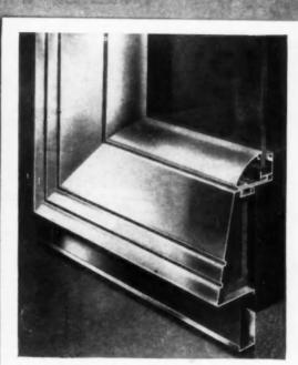
IN THIS NEW Pittco DeLuxe sill-sash combination, sill and sash are separate members, designed to be used together. Because they are installed separately, they reduce glass breakage. The Carrara Glass bulkhead is recessed, thus providing toe room and protection against breakage. This versatile new combination is invertible-may be combined effectively with any of the sashes in the Pittco DeLuxe line.
