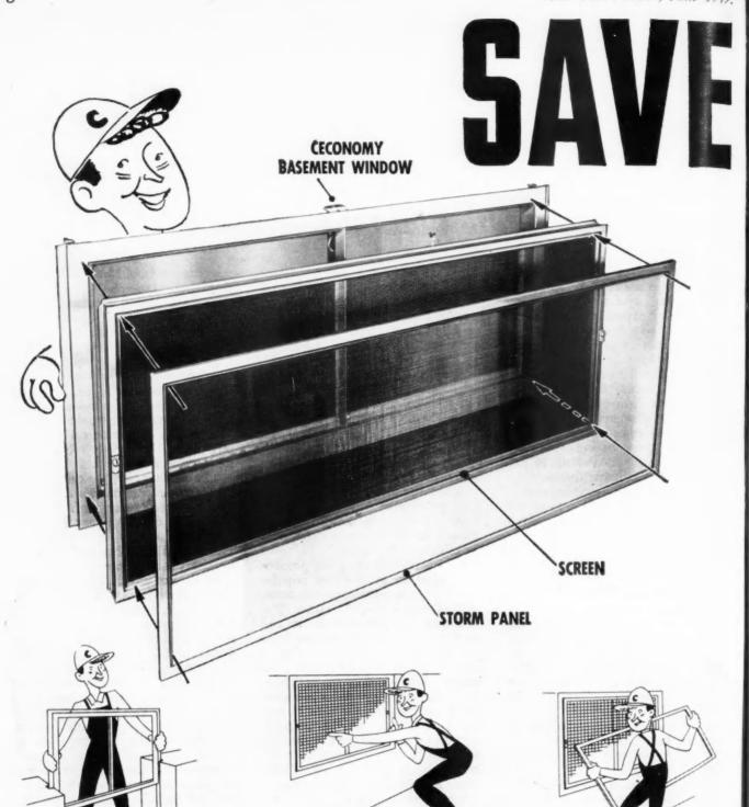
When you place your forms for the foundation, nail a wood strip on each side of your opening to provide vertical rebates. Strip forms, lower attached fins of Ceconomy Bosement Window into rebates. Plumb and level. Grout with concrete.
