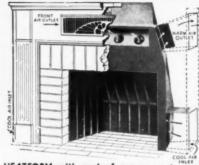
HEATFORM with part of masonry cut away
