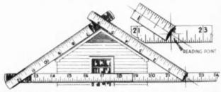
ROOF pitch can be measured from ground with triangle. Figure 2
