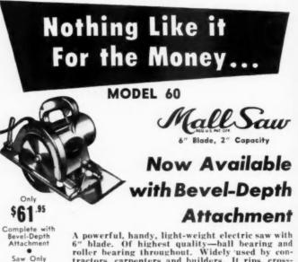
A powerful, handy, light-weight electric saw with 6" blade. Of highest quality—ball bearing and roller bearing throughout. Widely used by contractors, carpenters and builders. It rips, crosscuts, angle cuts rough or dressed lumber up to 2 inches. With Bevel-Depth attachment it will make straight cuts from 5/16" to 1-31/32" deep; and bevel cuts up to 45 degrees from 1/4" to 1-11/32" deep.
