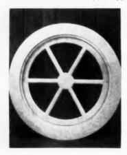
in Woodlife. Inner sash is a complete circle, with screen in upper half; sash ro-tates to provide ventilation. Operation is on a patented stainless steel weatherstripped track. Webb Manufacturing Co., Conneaut, Ohio.
