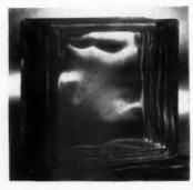
other places where decorative effects are desired. Random effect is achieved in production by use of several slightly dissimilar molds to form two halves of block, then using different combinations of halves. Designated as Insulux Glass Block No. 331. American Structural Products Co., Toledo, Ohio.
