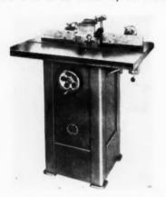
Shaper has three inch vertical spindle travel, with bearing assembly moving as a unit. Elevating is controlled by hand wheel and graduated dial; independently adjustand graduated dial; independently adjust-able guides are controlled by hand wheels. Motors are I HP single phase or II/2 HP three phase. Walker-Turner Div., Kearney and Trecker Corp., Plainfield, N.J.
