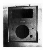
only; switch operated by hydraulic pressure changes in bulb. Specifications: 1500 to 4000 watts, 115 to 230 volts, 5122 to 13,660 B.T.U., 42 pounds in weight. All model WA-12 heaters fit same wall opening: 141/4 inches wide, 181/4 inches high, front plate 17 inches wide, 21 inches high, 53/8 inches deep and extending one inch from wall. Electromode Corp., 45 Crouch St., Rochester 3, N.Y.
