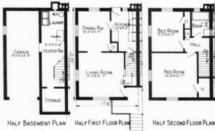
A HALF plan of each level of a compact typical duplex unit for an average family
