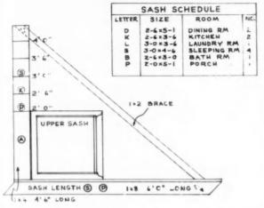
WHEN sorting sash for a number of jobs this builder found that it helped to make out a schedule of sizes, using the first letter of the room to designate where they occur. This letter is placed on the sash.
