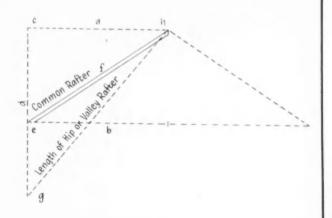
**T**HE above diagram indicates a rapid method of determining the length of valley or hip rafters after the width of building and roof pitch have been established.
