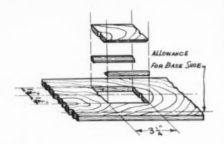
THIS is a simple method of cutting a hole in baseboard for an electric receptacle box.
