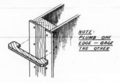
WITH the aid of plumb board, level the grounds on one side of opening and nail. Use the gauge to set grounds on other side. This will insure even spacing and eliminate plaster scraping when applying casings. Gauge can also be used in setting metal corner beads in arched openings. Any scrap piece of lumber can be used in making gauge.— Myron G. Miller, Williamsport, Pa.
