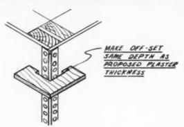
A SIMPLE method of installing metal corner beads is accomplished with the aid of a wood gauge. This gauge is made of a board 5 inches square and 3⁄4 inches thick. Cut out board in manner shown on drawing with offset same depth as plaster. The inside corner of gauge is pressed against the bead of corner bead with inside face of gauge placed against Sheetrock.—Myron G. Miller, Williamsport, Pa.
