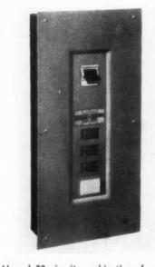
16 and 20 circuit combinations for either three or four wire service. Incorporates thermal-magnetic circuit breaker units that plug in on cylindrical bus bars and are interchangeable with those of NMO panelboard. Plug-in feature simplifies changes or additions of circuits when load increases are necessary. Underwriters' approved. Square D Co., 6060 Rivard St., Detroit 11, Mich.
