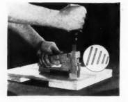
easy driving, this machine loads over a hundred lock-nails at a time that come nunarea lock-hails at a time that come adhered in one long strip for fast load-ing. Lock-hails are made in galvanized, copper, bronze or are electro-plated, in sizes from 7/16 to  $11/_8$ -inch long. The Heller Co., 2149 Superior Ave., Cleve-land 14 Chia land 14, Ohio.
