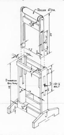
THE adjustable roller support is useful for handling long lengths of material after being run through a circular saw or joiner. The roller support is made up of various widths of three quarter inch and one inch stock as indicated in drawing. The roll is turned to a specific size; the  $\frac{3}{4}$ inch tension at either end can be made a part of roll or dowelled in place.—Elti J. Chiandussi, Youngstown, Ohio. American Builder, September 1949.
