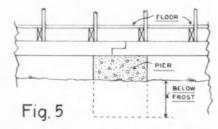
POUR concrete. After it has hardened remove form and take away the jacks. Pier must extend below the frost line extends below the frost line; yet, it is not unusual to find farm buildings resting on shallow foundations, or with sills precariously balanced atop boulders. Similarly, farmers know that run-off water can quickly pull soil away from and undermine foundations; yet, they fail to provide an adequate yard drainage system.
