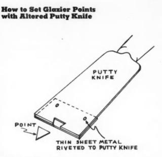
**B**Y altering the putty knife as indicated in the drawing a lot of time is saved in placing glazier points which are otherwise hard to handle.
