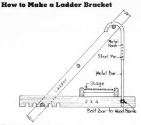
ADDER brackets may be homemade. A 2x4 and iron bracket are all that are necessary to make one. A 2x4 four feet long is sufficient to take care of most any pitch at which the ladder may be placed. Bolt two iron crossarm braces on each side of one end of the 2x4 horizontal member. The other end is notched to fit over the rungs of ladder. Flatten out the lower end of hook and drill three holes in same and equal distance apart. Bolt crossarm brace to hook and the bracket is complete.
