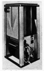
trapping of unburned gas. Incorporates snap-action thermal control automatic pilot and shutoff, Minneapolis-Honeywell thermostat, and combination fan and limit control. "Mono-Jet" single orifice burner is outside combustion chamber to prevent fouling from dirt or oxidation and is guaranteed for life. System measures 27x30x62 inches. Bard Manufacturing Co., Bryan, Ohio.
