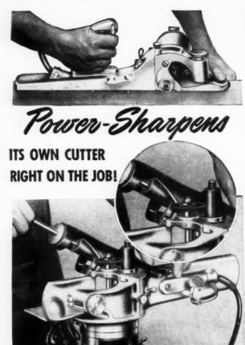
Keep your power plane cutter sharp on the job. You can resharpen the cutter in a matter of minutes, sharp as new. Just set the plane in the bench bracket, remove the cutter arbor and replace it with the grinding arbor and wheel. Mount the grinding attachment on the plane and switch on the power.
