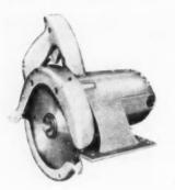
use on 110-volt A.C. or D.C. current, and delivers no-load spindle speed of 5,500 r.p.m. Weight, 91/2 pounds. May be op-erated with one hand, and aluminum motor r.p.m. housing makes convenient extra hand grip when desired. Stationary upper blade guard permits blade to be watched from either side while in operation. Black & Decker Manufacturing Co., Towson 4, Md.
