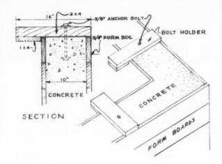
A NCHOR bolts can be held in position in foundation wall until concrete sets by means of short blocks with stop secured on one end.
