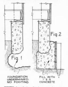
WHEN foundation footings wash away, walls settle. To repair, jack up sill, excavate under foundation, fill with concrete
