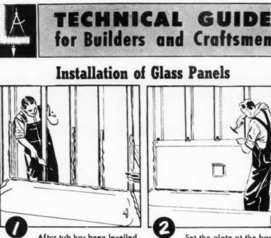
After tub has been levelled. place roll of mastic around rim for waterproofing. Also, butter studs with mastic before setting glass panels.
