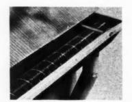
clogging gutters and leaders. Flexible 5foot sections of bronze mesh, internally supported by spiral brass spring, are laid full length of troughs, insuring free drainage and repelling foreign material. Leaves blow off or are kept dry until they disintegrate. Standard 3-inch diameter tube fits any gutter up to six inches. Gutter Screen Manufacturing Co., 80x 447, Newark, N.J.
