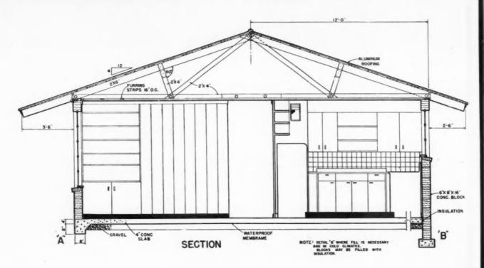
thick insulation. There are aluminum louvers at gable ends and screened vents between rafter at wall. Windows are aluminum, with tile sills.
