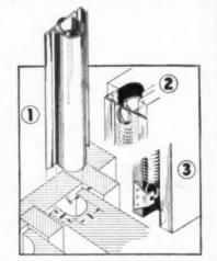
balanced with coil spring tension and metal housing tension, providing fingertip window control. In raising and lowering sash, spring housing compresses against groove for stability, but does not hinder vertical movement. Coil is concealed in flexible tubular metal housing in ½x½-inch sash stile groove. Allmetal Weatherstrip Co., 2241 N. Knox Ave., Chicago 39, III.
