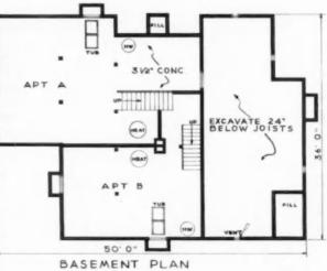
EACH unit in duplex apartments has individual basement with its own heating plant and laundry trays. Ranges and refrigerators are included in rentals
