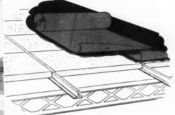
SIMPLE EASY CONSTRUCTION — Sub-purlins are installed, Kaylo Tile laid, end joints grouted and roofing material applied—that's all there is to this better roof deck. No special tools or skills needed. Kaylo Tile can be sawed, shaped and nailed with common tools.
