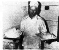
MUCH smaller volume of sand plaster, right trowel, equals the weight of perlite
