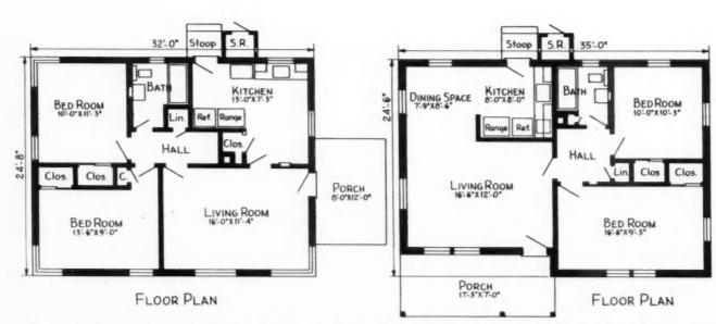
TWO and three bedroom homes are built on concrete slab with footings under exterior walls and interior load bearing walls.
