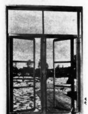
Suitable for all residential construction, frame, masonry or brick veneer. Stool, head and jamb sections formed from 18-gauge steel, bonderized and primed. Easily assembled by steel tenons, which are ex-tensions of head and sill members inserted in slots in jambs and bent into holding position. Angle fin provided, if necessary for structural requirements. Hope's Win-dows, Inc., Jamestown, N. Y.
