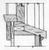
FRAMING for typical window introduces a sployed sub-sill on which the regular sill of window frame is placed. Sub-sill provides solid sulling for stool and appear
