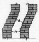
A COMMON structural fault which presents flue venting difficulties is on inversertly-built chimney offset. It corhelling is hegun on both sides of flue at the same level, diameter of the offset section (B) will be less than diameter of straight run (A). This creates α bottleneck, restricting the volume which the chimney will handle
