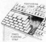
IN APPLYING esphalt shingles over an old wood shingle roof, first notil down all loose shingles. Split warped shingles and notil down the segments. Place bevelled wood "leathering strips" along the huts of each course of old shingles. Then apply an eaves floshing strip of esphalt roll roofing along the eaves. Use six notik in each three-toh, square butt, asphalt stripshingle.
