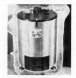
leaving only fine ash automatically swept into large ish drawer. All accessible outside surfaces are insulated with one inch of asbestas. Dimensions are height-36 inches; diameter-24 inches; A y-inch gas connection and a five-inch flue are required. Autogas Company, Dept. A8, 2153 W. Fullerton Ave., Chicago 47, III
