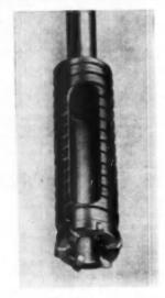
pirot, new drill penetrates concrete at speeds up to six inches per minute with less pressure than required for ardinary drills. Attevized core particles escape through side exhaust tiet. Used with andinary electric drills at speeds from 500 to 1200 r.p.m. Drills up to 30 feet without resharpening. Tilden Tool Manufacturing Ca., Dept. A8, 1995 N. Foir Oaks, Pasadena 3. Calif. (Continued in page 142)
