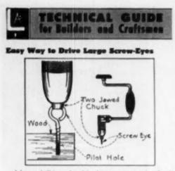
A breast drill is used to drive large screw-eyes into hardwood material. Undersized holes are first drilled as a starter. then the chuck of drill is placed over large screw-eves as illustrated. Chuck is then released after screw-eye is in position .- Submitted by Herbert E. Fey, New Braunfels, Texas
