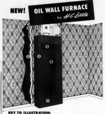
1-FURNACE is 80" high, 20" deep, 30" wide. 2-PARTITION wall cut away shows how furnace is set in wall to extend out equally each side (7" for a 6" wall) 3-FURRED OUT wall above furnace both sides provides ample room (20" x 30") for a 4-PATENT FLUE, which comes down from above. (Or brick chimney constructed at side may be used) 5-WARM AIR discharge grilles, 8" x 27", both sides. 6-BADIANT PANEL, 12" x 49", one side. 7-COLD AIR intake grilles, 10" x 27", both sides.
