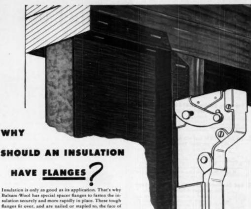
Balsam-Wool has special spacer flanges to fasten the insulation securely and more rapidly in place. These tough flanges fit over, and are nailed or stapled to, the face of the framing members. Proper air spaces, one on each side of the insulating mat, are also provided by these flanges. The result: a sealed, tight, foolproof application for maximum Balsam-Wool insulating efficiency!
