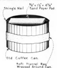
Use an old cuffee can for this purpose. Glue a sandpaper pad to piece of wood, drive sluingle nails on both ends of can as shown, and a place for pencil shavings and lead has been arranged. Wrap a soft flaimel rag around the can and wipe pencil points after sanding.—Submitted by J. G. Caldwell, San Mateo, Calif.
