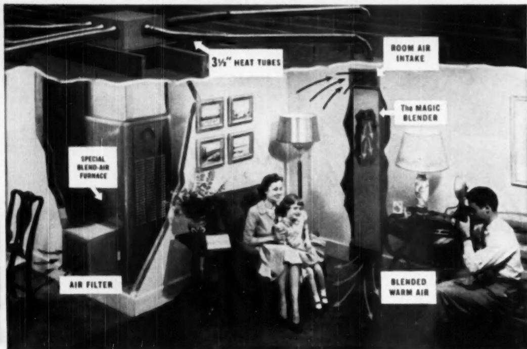
This illustration shows a Coleman BLEND-AIR installation with the furnace located in the utility room. The Heat Tubes are located in the attic. In basement installations, the Heat Tubes are located in the basement immediately beneath the floor.
