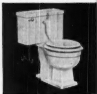
PRINCE VITREOUS CHINA CLOSETS —For 12-in. roughing-in. Round front extended shelf bowl. Reverse trap close-coupled combination, free-standing model. B-6420 (illustrated).
