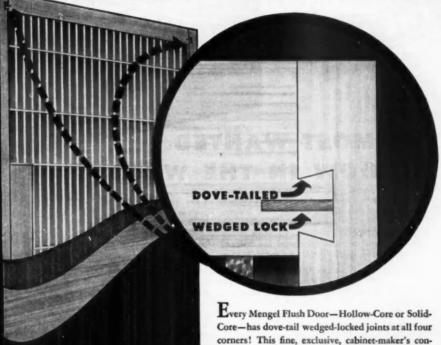
Every Mengel Flush Door—Hollow-Core or Solid-Core—has dove-tail wedged-locked joints at all four corners! This fine, exclusive, cabinet-maker's construction is found only in Mengel Flush Doors—requires more lumber, extra machining and labor, but you get stronger and more stable doors.
