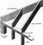
ORDINARY 2x8 jack raiters should be nailed to hip rafter with three 10-penny nails
