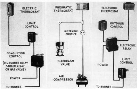
THREE basic types of heating plant control—electric, pneumatic and electronic—are outlined above
