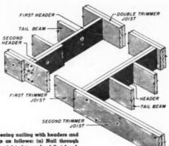
FLOOR opening nailing with headers and trimmers is as follows: (a) Nail through first trimmer joists into ends of first headers with three 20-penny nails. (b) Nail through first headers into ends of tail because with three 20-penny nails. (c) Nail second headers to first with 16-penny nails spaced six inches longitudinally and placed near top and near bottom. alternately. (d) Nail through first trimmer into ends of second header with three 20-penny nails. (e) Nail second trimmer joist to first
