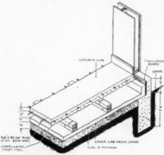
SECTION of floor showing 3-inch concrete slab over slag fill, and corrugated steel resting on brick baffles to support upper 3-inch heavily reinforced concrete slab
