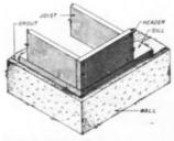
THE HEADER joist should be nailed to the other joists with 20-penny nails—three to the end joist and two to the others. The end and header joists also should be toenatied to the sill with 10-penny nails spaced approximately 16 inches on center
