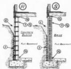
VARIOUS types of foundation walls shown above, with the 1-2-3-31/2 fundamental steps of the standard specification. which control the infiltration of termites into an existing or new building
