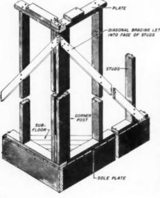
THE LOWER part of the top plate is nailed to each stud and corner post with two 16penny nails. The up per half of the plate is nailed to the lower with 10-penny nails. two near the end of each piece, the others staggered 18 inches apart. Corner braces are fitted into notches in faces of framing members and natled at each stud with not less than two 10penny nails, and at ends with three 10penny nails
