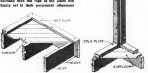
THE SOLE plate is nailed through the subfloor to header joists and regular joists with 16-penny nails staggered as shown. The sole plate over the end joist is nailed through the subfloor to the joist with 16-penny nails spaced 16 inches on center. For nailing plates on which raiters bear, see drawing on the next page
