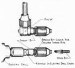
To use old bits with electric drill take bit brace apart at the ratchet. By placing the round shaft through the ratchet of drill chuck and placing the square bit shank in the brace chuck, it is possible to use square and round shank bits in the drill.
