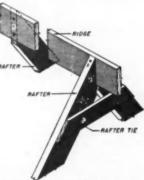
THE RIDGE (a) is natiled to the first ratter of a pair with two nails (16-penny for 1-inch ridge or 16-penny for 2-inch ridge). The second ratter (b) of a pair is natiled through its top edge to the ridge with one 16-penny nail and toenailed to the ridge with one 16-penny nail. The ratter tie or collar beam (c) is natiled to each ratter with four 10-penny nails
