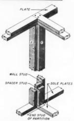
IN CONNECTING a partition to a wall, the upper member (a) of the partition plate is natised to lower (continuous) member of wall plate with two 16-penny nails. Wall studs (b) are nailed to the spacer stud will 16-penny nails 12 inches on centers. The end stud (c) of the partition is nailed to the spacer stud with 10-penny nails staggered with about 12 inches between the nails
