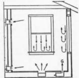
PERIMETER floor delivery at G with return at B or D. Warm air covers windows
