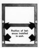
No Head or Side Room Necessary—The small diameter of the new negative spring cuts the balance size by 75%, thereby allowing the Powerful Pigmy to be mounted in the window sash itself. This is the first time in residential window history that a true counterbalance is available which requires neither head nor side room. It is the greatest innovation in balancing double hung windows since the spring balance was developed by Pullman over 65 years ago.
