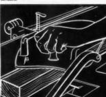
Bevaling — Big tables, designed for simple accurate depth adjustment. This operation shows bevoling at 45°, Fence may be tilted to 45° in either direction.
