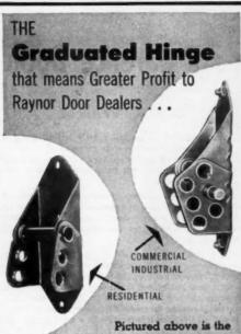
Pictured above is the Patented Raynor Graduated Hinge. By inserting the track foller in the special hole for each section the Graduated Hinge, combined with a tapered track, produces Raynor Graduated Seal.
