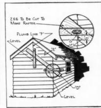
For the novice who is not familiar with the standard method of determining the pitch of roof rafters and how to cút them, the sight method shown in sketch will suffice.
