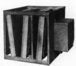
traps even the smallest dirt particles. Automatically cleaning the air by electrical attraction, the Magne-filter effectively removes pollen, air-borne bacteria, dust, and smoke. The Magne-filter is designed to be installed in the return duct of the air conditioning system, and can be installed on its side in limited space applications.
