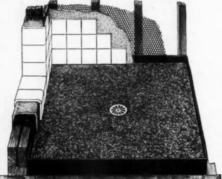
Details of suggested construction in building up a tile shower on a Fiat precast receptor. Metal lath and foundation plaster are brought down inside the rust-proofed metal flange. The tile setter starts directly with the wall construction without the delay involved in laying a tile floor and waiting for it to harden to a working surface.
