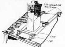
When chimney repairs are necessary, the scaffold for doing the work may be easily made from ordinary lumber which is not too heavy in weight or too hard to work. With the device shown in the sketch, access to all four sides of chimney is possible.—Arthur N. Nelson, Kansas City, Mo,
