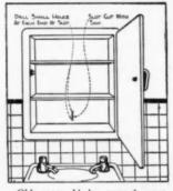
Old razor blades may be permanently disposed of by cutting a slot in the rear wall of the medicine cabinet. Bore two small holes at each end of the slot. A keyhole saw is then used to cut out the slot. If cabinet is made of metal a hacksaw blade cut to narrow point at one end will be required for sawing the slot.—Arthur N. Nelson, Kansas City, Mo.
