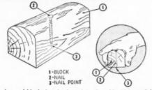
A wood block that fits into the palm of hand is used for a board pusher. (1) Smooth the top edges of the block. Drive nail (2) through center of block so point (3) extends  $\frac{1}{2}$  inch from block. File nail sharp. Board on saw table slides easily using pusher.—Warren W. Howe, Longview, Wash.
