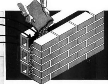
Cavity Wall is a new type of *insulated* wall which requires no furring or lathing. It can be plastered direct, or interior masonry surfaces may be left exposed.
