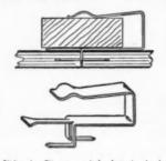
Sliding Loc-Clip, new unit for fostening insulation board tile to furring strips, eliminates the need for harmer or naits. It will work with T. G or square joints. Designed for 1x2-inch furring strips. Just put on the market by E. G. Building Fasteners Corp., 101 Park Ave., New York 17, N.Y.
