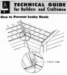
A low pitched roof joined by a valley to a roof of much greater pitch often has a tendency to cause trouble due to rain water seeping in under the shingles of the roof of lower pitch. This can be corrected by providing a standing seam of galvanized iron in the center of valley as indicated in the drawing above.—Submitted by H. W. Greiner, Landisville, Pa.
