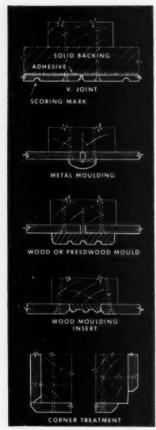
VARIOUS joint treatments may be used between hardboard panels. A slight space between panels is recommended
