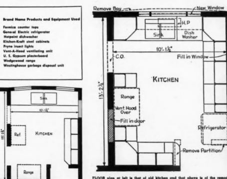
FLOOR plan at left is that of old kitchen and that above is of the remodeled kitchen. Note arrangement of all equipment for maximum efficiency in use
