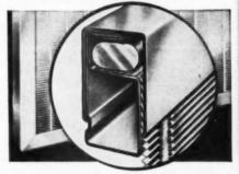
KAISER ALUMINUM SCREEN FRAME is readily assembled from framing sections, trim cover sections and cast aluminum corners. When framing Kaiser Aluminum Shade Screening the spline is used only at the top and bottom of the screen. No screws are needed. The frame may be used with conventional wire cloth screen as well as Kaiser Aluminum Shade Screening.
