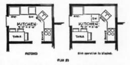
In setting up the proper equipment for a kitchen such as the one diagrammed in Plan No. 3, the architects selected a drop-in-dishwasher of the top-opening type, as shown in the Preferred sketch [illustrated above]. The second sketch indicates that the front-opening model is not a good choice because in an open position it would prevent easy access to the sink.
