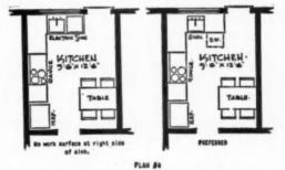
Plan No. 4 also shows a kitchen in which the greatest need is for counter space, on both left and right sides of the sink. A front-opening washer is the better choice; with a top-opening model there would be no counter space on the important right side of the sink.
