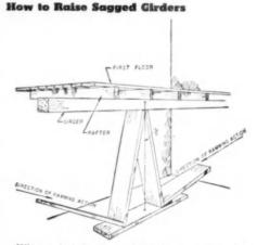
When a jack is not available the method of raising sagged girders as indicated in sketch above can be adopted. A 2 x 10 sleeper 8 feet long is placed on the floor under the area of the girder to be raised. Two 2 x 10 shore members are placed diagonally under the girder and on sleeper. Place 2 x 10 rams on each side. With two men ramming the shore members at the same time girder can be brought into position quickly.—James T. Strahan, West Collinswood, N. J.
