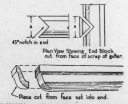
TO PROVIDE a moulded closing end of the gutter a 45 degree notch is cut in the end to be closed and a segment fitted into it. The triangular section is cut from small scrap ends of gutter
