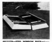
AB123/Y-SIEk VINDW BUCK tewas. nee Mig. Co., Dept. AB, Kewanee, III., For initaling basement windows in poured concrete foundations, this buck produces a clean finish around the window, eliminates leaky montar joints at sill and jambs, installs every window frame square and true. Photograph shows buck open, with window frame inserted. Buck is then closed and tightened with wing nuts, being then ready to be fostened to form wall. Buck is stripped off when forms are wrecked. Booth 216, Stevens
