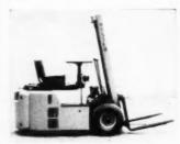
AB12289—LIFT TRUCK—Hyster Company, Dept. AB, 2902 N.E. Clackamas Sr., Portland B, Ore. Company reports engineering changes in Hyster's Model '20' lift truck are a new upright assembly and new load arm pins which will permit the use of optional additional counterweight on the standard 2000 pound capacity model, (shown above thus increasing or decreasing loadcenter or load capacity as the need requires. Photo shows extra demountable counterweight "pads on back.
