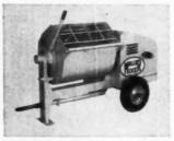
AB12114-PLASTER MIXER—Muller Machinery Co., Dept. AB, Metuchen, N. J. The 3 cubic foot plaster and mortor mixer recently introduced by Muller, is now equipped with a neoprene seal to eliminate wear on the paddle shaft. The small Muller mixer is built long the same heavy-duty lines as the larger machines, according to the company. Convenient loading height is 32 inches and a width narrow enough to go through a 30-inch door. Also available in 6 and 9 cubic foot sizes. Gos or electric powered.
