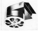
AB12131—VENTILATING FAN — National Appliance Co., Dept. AB, 4814 W, Vernor, Detroit 9, Mich. Model 30:C Ventrola ceiling fan shawn will move 500 cubic feet of free air per minute. Ceiling opening is 11½, inches; connectstructed so that standard 3½ x 12 inch furnace pipe may be used. Two unit construction permits installation of grille, motor and blade after placing of sleeve and shutter. Blade size, 10 inches; speed 1600 r.p.m.; watts 42. Approximate shipping weight, 20 Ibs.
