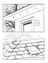
If the roof has large overhangs ventilation can be secured by cutting holes into the underside of the soffit. These will need screening to keep insects from entering the house. Small, metal louvers of 3-inch diameter are manufactured for this purpose and are easy to install. If the roof does not have any overhang then a roof type ventilator can be installed.
