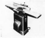
AB12106—POWER JOINTER—Delta Power Tool Division, Rockwell Mfg. Co., Dept. AB, Milwoukee 1, Wis. One HP eight-inch Delta jointer deep and makes 16,400 cuts per minute at 4100 RPM. The 30-inch-long front table and 30-inchlong rear table have a width of 9% inches. Precision fence tills 45 degrees right and left for auck adjustment. Safety cutter head is equipped with four knives and is copable of a three-inch cutting circle. Swing-out safety guard covers blade at all times. Booth 13, Stevens.
