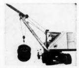
THE CRANE ADAPTOR shown above converts back hoe machine to crane in five minutes on the job. is used for low-ering pipe or valves into the ditch. and is interchangeable with a fast back-fill blade using same boom and sitck
