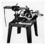
RADIAL ARM FOR MOUNTING ELEC-TRIC HAND SAWS has cut off movement of 24-inches. Bevels or miters 0 to 45 degrees left or right, 9% inch vertical adjustment
