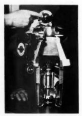
CUT.AWAY MODEL OF NON-CLOGGING DISPOSAL UNIT with shredding mechaniam which reduces refuse to small particles. Sink cover can be used to start mechanism. or used as sink stopper or strainer
