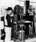
BAND SAW above has a built-in guard. Only required sawing portion of the blade is exposed. Table adjustments are provided, and anti-friction guides reduce saw blade steel crystallization
