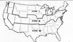
Figure 6.—Condensation zones.—Zone I roughly includes the areas with design temperatures -20° F. and colder; zone II 0° to -10° F.; and sone III areas warmer than 0° F.
