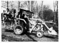
COMBINATION TRENCHER and front end loader. This machine is used for digging foundation walls, footings, sewer, water lines
