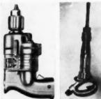
POWER DRILLS are available in a variety of sizes and types. Right, is shown low speed, lightweight drill geared down to 450 r.p.m. for drilling steel, glass, brick and other hard materials. Left is drill-hammer for masony. The bit both hits and rotates at the same time, and has '4 to '34-inch drill capacity
