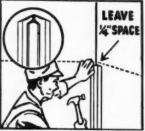
FIG. 7—Install vertical metal mouldings. Keep top end of moulding ¼-inch below level line and allow enough space at bottom of vertical moulding for base moulding to fit neatly below it. Mouldings are nearly always recommended and must be used wherever moisture is present
