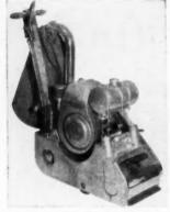
HEAVY DUTY FLOOR SANDERS using a revolving drum to which sandpaper is fastened. Finishing or refinishing may be done cheaply with modern sanders
