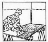
PIG. 9—Cover the entire back of the board with cement, spreading it generously with a toothed trowel. Start applying the board in one corner at wainscot level and continue around the room to door opening. Then proceed from the same corner, in opposite direction, to the same door opening. Press the board firmly to the wall, using a few 1/4-inch brads to hold it in place until the cement sets
