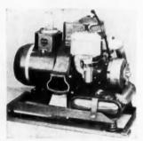
PORTABLE ELECTRIC GENERATORS provide power for saws, drills, and other tools on the job. Unit shown can be carried by one man, is spring mounted to reduce vibration
