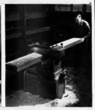
JOINTER The long work table on the Delta 8" Jointer makes it an ideal tool for easy handling of long boards. The special 4-knife cutter-head is 33½ per cent faster than a 3-knife machine. Making true "finish" cut fast eliminates extra operations. Also available in 6" model.
