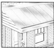
Porch roof—vertical and horizontal seams are flat locked.
