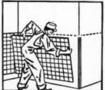
FIG. 8—Cut the hardboard with a fine tooth crosscut saw and sand edges before fitting and installing. Bevel back edge of board slightly for perfect fit. Scored edges of the board should always be kept to the top and right.
