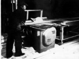
RADIAL SAW This new 16" Delta Radial Saw cuts through the entire 360" at every conceivable angle. All cuts are made above the work table, in clear view. For miter capacity and extraordinary versatility, this saw truly has no equal. Also available on 8", 10", 12" and 14" models.
