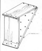
This is a bracket that can be picked up and placed anywhere on the roof in the process of applying roof boards or shingles. The bracket is made of 34 inch thick material and of shape to fit the pitch of the roof. Through the bottom member drive several 1½ inch roofing nails so the points show about 3½ inches. This will keep the bracket from sliding.—John Menkveld. Grand Rapids, Mich.
