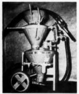
THIS CONCRETE APPLICATOR has a dual-compartment pressurized hopper for continuous operation. Adjustments for air and water pressure can be made while the unit is in operation, and different materials can be handled without changing parts.
