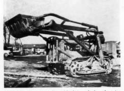
CLETRAC, equipped with ¾-yard bucket, used where the going gets too tough for the "scoopmobiles." It also has a blado attachment so that it can be used like a bulldozer for light grading work
