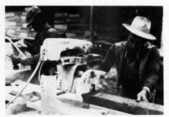
ABRASIVE stone wheel makes clean, fast cut
