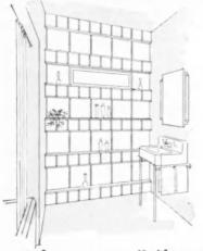
Bathroom exterior wall. Alternate horizontal courses of 6" and 12" glass blocks staggered with horizontal wood shelves between. Stock ventilating sash is set in 12" row between 5' and 6' level.
