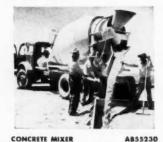
Plus Mix models of new mixers are a development of Jaeger. The unit is adaptable to varying conditions among ready mix operators. The new units are available in 3, 41/2, and 61/2 yard capacities. Many choices of equipment are available with the mixer. Jaeger Machine Co., 500 W. Spring St., Columbus 16, Ohio.
