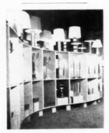
PLASTIC-FACED PLYWOOD was used to good decorative effect in these display fixtures for Westwood Industries. Paterson. N. J.. lamp manufacturer. The material is GPX. manufactured by Georgia-Pacific Plywood Co.: the plastic overlay does not mask the grain of the Douglas fir beneath it
