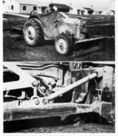
(TOP) EASY MANEUVERABILITY of this two-bladed Fordson tractor fine-grades lawns economically. (Bottom) ripping claws attached to the blade of a Caterpillar doser is an invention of the Denver concern. The close-up photo shows how reversing the machine rips the earth and makes dosing in hard or frozen ground easier. Normally, claws are in a raised position
