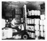
PALLET LOAD OF NAILS is removed from storage. Truck has 4.000 pound capacity
