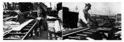
REAL MONEY MAKER is the upgrading operation where millrun lumber is used instead of shop grade lumber. Scraps are used for shingle backers. Machine is an "XL" ripper JUMP SAW is used for the length upgrading operation. Here workman cuts out clear span of lumber before sending to the mill. Machine is a Superior Speedster 8-inch jump saw
