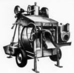
Jacger 31/2 S "Auto Looder": Mixes 12 to 15 more yds. of concrete a day because it can be loaded while previous batch is being mixed, then hopper automatically shakes load into drum in a flash. Jacger engineered for long life. Machined steel drum tracks ride on carwheel rollers, Automotive transmission.
