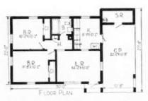
TWO-BEDROOM FLOOR PLAN features compact room arrangements with little lost space. Both bedrooms have steel, sliding-door wardrobes. Storage and utility room is located at the rear of the carport.
