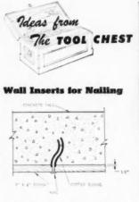
Short lengths of copper tubing are inserted into concrete wall or mortar for future nailing of boards to the surface while the mix is still wet. Tubing should be selected that will admit the nails that are to be used. Cut tubing into 4-inch lengths and bend into an S-shape as shown. When the board is to be nailed in place, hold it against the projecting tube and tap with a hammer to mark the reverse side. Drive a nail through board to mark position.—Herbert E. Fey, New Braunfels, Texas.
