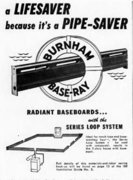
Save pipe? You bet! A good fat 40%. Why? Because when you hook up Burnham BASE-RAY® Radiant Baseboards in the Series Loop System (shown above) it actually becomes part of the main. Just a glance at the diagram shows how it saves scarce pipe. And better still this foolproof system saves you 49% in fittings and 54% in installation labor costs. In these days that's to the good and remember you're giving your customers a modern radiant heating system to boot. •Reg. U.S. Fat. Off.
