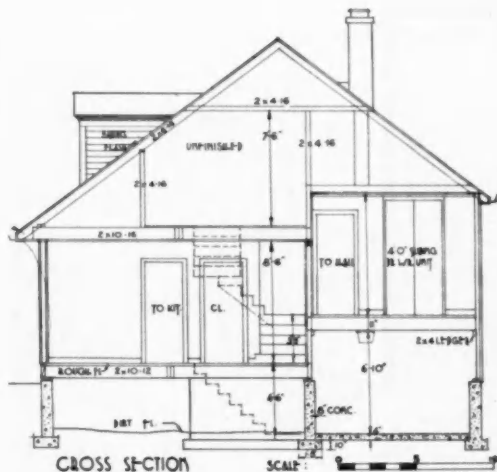
First level has kitchen and living-dining room. Bath and two bedrooms are on the second level. Plumbing is back to back
