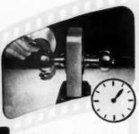
STEP ONE ... After releasing the inside turn button, the hidden pin is depressed with a pointed instrument, unlocking knob from the lockset.
