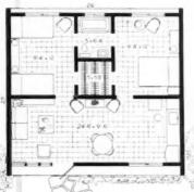
MODERN CONSTRUCTION - built on concrete slab, standard \* frame construction, two outside masonry walls, flat deck roof, stock millwork throughout, engineered for livability and comfort.
