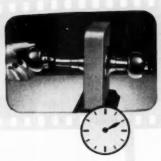
STEP TWO... Here is the knob assembly, containing the lock guide sleeve and the cylinder, being removed as a unit from the spindle.
