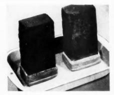
keep both brick for a few weeks in a shallow pan of water, as shown. Try this with Brixment mortar!
