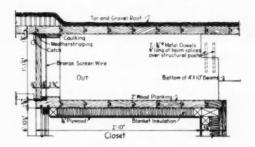
Screened opening allows air to enter the quest room. Closet coiling is lowered to form the duct. Ventilating panel over doorway is raised and lowered with the aid of  $\alpha$  dowel rod attached to the transom catch
