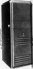
▲ COUNTERFLOW-PURNACES. For small basementless homes, especially those using perimeter beating systems. Three sizes with capacities from 75,000 to 125,000 Btu. Height is 83 inches, depth 29 inches, with widths varying from 12 to 23 inches.
