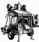
Jueger 31/2 5 "Auto Louder": Mixes 12 to 15 more yds. of concrete a day because it can be loaded while previous batch is being mixed, then hopper automatically shakes load into drum in a flash. Jaeger engineered for long life. Machined steel drum tracks ride on carwheel rollers. Automotive transmission.
