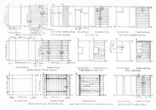
FIG. 4-Various types of strapping conditions
