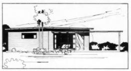
Combination rafter-joists give pitch to the roof and a level ceiling in this elevation. This is made possible by ripping 18-toot 2x14's diagonally to get two 18-toot pieces 4 inches wide at one end and 10 inches at the other. The 10-inch widths are placed at the ridge
