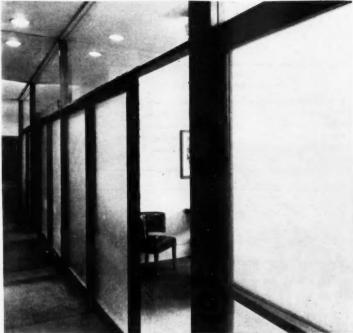
Mirror covers wall at end of corridor down row of private offices, heightening sense of space for an interior of limited area. Glass in wall panels has a smooth surface on the corridor side
