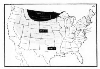
Three-sone map showing regions where gypsum sheathing may be used to meet minimum FHA heat loss requirements in various parts of the country. Gypsum sheathing costs are within 514.714 cents per square foot according to zone location
