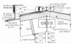
Anchor detail. Two sections are bolted together in 12 places
