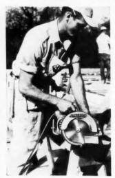
The new Dual V-Belt Drive eliminates gears-provides shockabsorbing, velvet smooth operation for faster, cleaner cutting. Cuts and rips wood; cuts and scores brick. tile and other materials with 6000 RPM full load blade speed. Its high speed feeds the blade in-no need to push or ram. The powerful motor-full ball-bearing . . . exceptionally cool-develops up to 1-1. H.P. It weighs 19 lbs., just the right weight for its 8-1/2" blade and 2.11 " cut.
