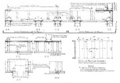
FIG. 5—Typical ceiling details
