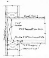
FIG. 1—Typical section through exterior wall where dry wall construction is used. Note position of 1x3 starter piece strapping
