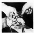
vides leverage during the application and is snapped off leaving a neat slice with no sharp ends. The small diameter of the connector adds but a fraction of an inch to the diameter of the wires. The small unit is valnable for joining wires in crowded junction boxes.
