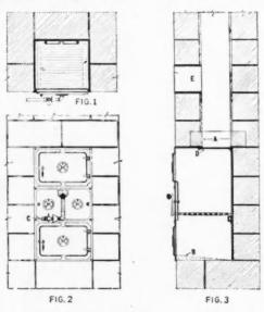
finish floor. Heating plant flue or separate flue location is used. Fireplace flue ash drop is never used. As in Fig. 3, flue tile is placed directly over the opening in the top of the incinerator. Firebrick is used as indicated at point "A" if necessary to avoid extra cutting. The block voids are filled and a cement or mortar ash pit floor is grouted in, as shown at point "B". The unit must be set so that there is a smoke-tight seal between the incinerator and the flue (point "A").
