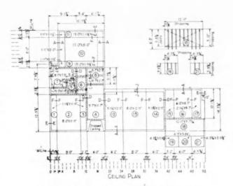
FIG. 3—Ceiling plan showing joist framing in two directions
