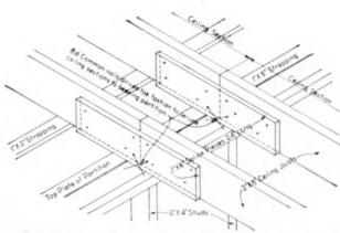
FIG. 2-Joists butted over bearing partition and spliced by 2-foot "one-by" boards
