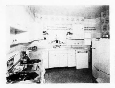
The service porch was eliminated in order to make a large room. The hot water heater was put into a closet. This job used Geneva cabinets. G.E. Monotop. Dishmaster. Armstrong spatter linoleum. Sherwin-Williams washable wallpaper, Coralite on two walls and ceiling. Bendix washer. Cost was about \$3.200
