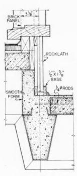
Section through window to roof deck
