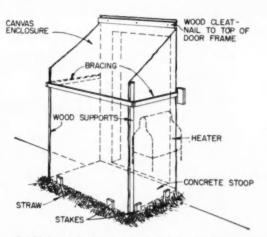
Portable heater placed in the doorway protects stoop when poured in winter. Canvas canopy is placed around form and attached to doorway
