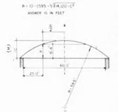
The dimensions on the drawing are for the specific points on the truss as requested. The formula of h  $\sqrt{R^2 - {2 \choose 2}}$  R-H will apply to h value for any point along the truss, h height at any particular point along the top cord of truss.
