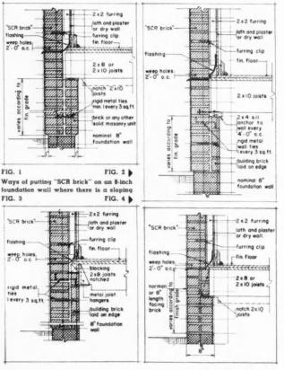
Beginning a series of solutions to building problems encountered in using the new "SCR brick" on the job
