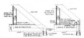
FIG. 4—Section through knew wall in dropped plate condition (left) and with raised plate. Knew wall height (H) is the combined height of knew wall section plus inside face of the beveled purlin above it
