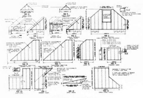
FIG. 2-Standard non-rectangular wall sections
