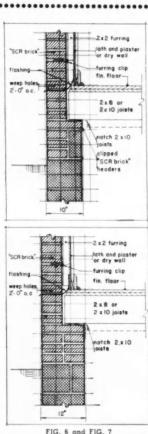
Two typical details for the use of "SCR brick" walls on 10-inch and 12-inch foundation walls
