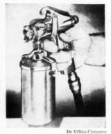
PAINTING WITH SPRAY GUN. Finger-tip adjustment control quickly provides a wide selection of spray patterns for various types of jobs and paint materials.
