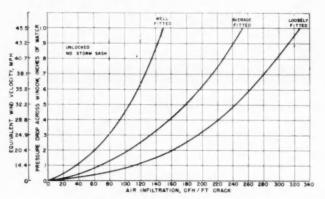
Figure 15. Infiltration for Non-weatherstripped Windows
