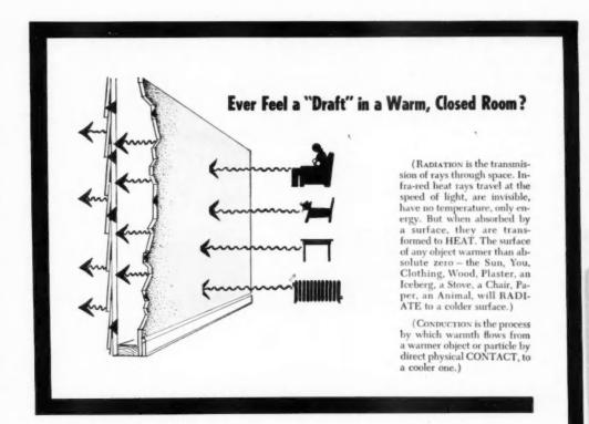
People often complain of "drafts" in a room with air-tight walls and windows. Why? To a large extent because, by Nature's law, warmth *flows* to cold by RADIATION as well as by CONDUCTION. Cold walls, too, draw heat out of contacting air by conduction, causing a downward current of cold air.
