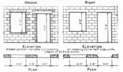
Right and wrong methods of planning concrete block masonry walls. The correct method utilizes full size units. The mason does no cutting. Savings can result for the builder
