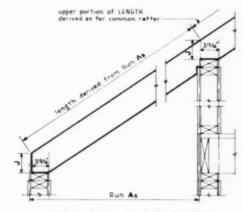
FIG. 5-Rafter with double bearing
