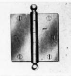
AB13315—BOOTH NOS. 275-276—BUTT HINGE—C. Hager & Sons Hinge Mfg. Co., 139 Victor St., St. Louis 4, Mo. The model No. 1241 Full Mortise Butt Hinge illustrated is designed for general interior application on doors of residences and other medium weight doors receiving average service. Hinges are furnished either with ball tip or button tip; they are made of wrought steel in nine different finishes. Recommended for use where a high grade of hardware is desired.
