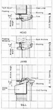
FIG. 12-Modular wood casement window detail
