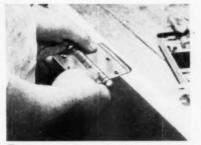
"The butt itself is perfect. There's no splitting of the wood, no rough spots. It's the right depth and size so the hinge snaps in without further work."
