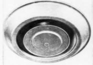
AB13310—BOOTH NO. 645A—AIR DIF-FUSER—W. B. Connor Engineering Corp., Dept. AB, 500 Fifth Ave., New York IB, N. Y. Stripped of non-essential controls, this unit is designed for homes, while retaining performance characteristics of industrial models. An inconspicuous dome-shaped outlet, it consists mainly of a collar and an inner and outer deflector. Inner deflector is positioned so that air is discharged outward and downward; outer deflector further diverts air from adjacent ceiling area.
