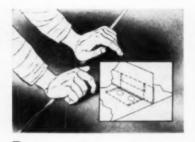
5. The top half inch of the one-inch flange on the second strip is bent down over the top of the half-inch flange of the initial strip
