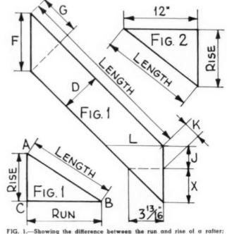
FIG. 1.—Showing the difference between the run and rise of a ratter; also some important dimensions in rafter cutting
