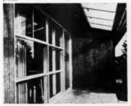
AB13038-BOOTH NO. 16-EXTERIOR SIDING-Johns-Manville Corp., Dept. AB, 22 E. 40th St., New York 16, N.Y. Color and pattern are incorporated into a large size asbestoscement sheet for exterior siding. The "Color-bestos" sheets, 32x96 inches by approximately 3/16 inches, provide weather and fire protection, and can be used effectively on the soffits of overhangs, as above. Seven colors, made up of tiny ceramic granules are provided. The randomribbed pattern makes joints and nail heads in conspicuous
