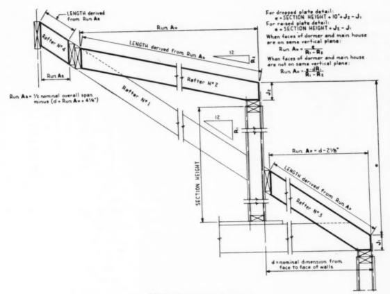
FIG. 7-Shed dormer roof rafters
