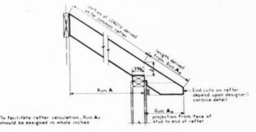
FIG. 4-Common rafter with overhang
