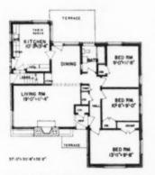
Massive fireplace and kitchen receive the emphasis in this Detroit house. The kitchen is enlarged to include a breakfast area, yet the house has a separate dining room. The house is of brick veneer construction with a full basement. The dining room opens to a terrace for summer use.
