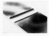
**11.** Trim the corners on the flanged end of each strip sufficiently to clear the end flange and the side flanges. This is indicated by the intersection of dotted lines shown in sketch above where two separate strips are placed
