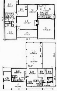
The Flexabilt house features movable storage walls and air conditioning. It can be converted from a one or two bedroom unit into a three or four bedroom unit or a two bedroom house with an efficiency apartment.
