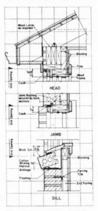
FIG. 1-Standard modular double-hung wood window detail with patented side balances
