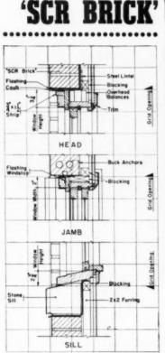
FIG. 11-Modular wood double-hung window detail with overhead balances
