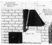
AB13188—FIREPLACE DAMPERS—Superior Fireplace Co., Dept. AB, 1708 E. 15th St., Los Angeles 21, Calif. Adaptable for fireplaces with openings on front and sides, or opening into two rooms, the "Hi-Form" damper guarantees the proper construction of the fireplace throat. It serves as a guide, around which the masonry is built. The damper, when in open position, does not swing back beneath smoke flue, preventing downdraft winds from entering the throat, forming a perfect draft for the fireplace unit.
