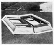
AB13054—BOOTH NO. 284—STEEL WIN-DOW BUCK—Kewanee Manufacturing Co., Dept. AB, 150 Burlington Ave., Kewanee, III. This device is used to install steel basement windows in poured concrete foundations. Its use eliminates the need for wood forms and gives a cleaner finish around the opening. The buck does away with leaky mortar joints at the sill and jambs. Two perforated straps on each side of the buck permit it to be nailed or bolted to forms on either the inside or outside of the basement wall.
