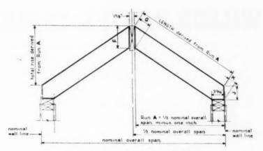
FIG. 3-Details of common rafter calculation
