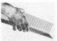
AB13198—BOOTH NOS. 29-30—METAL LATH—National Gypsum Co., Dept. AB, 325 Delaware Ave., Buffalo 2, N. Y. This smoothedged metal lath product is stated to assure lath installers and warehousemen freedom from cuts and scratches. It is used to reinforce plaster and prevent cracks at all interior corners. Called "Safe-Edge Cornerite," it is mainly applied over gypsum lath. It is smooth-edged and formed at the factory, Smooth surface speeds plaster application and cuts waste. Available in two sizes.
