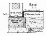
cast. Further tests by the University of Michigan show the material to have a four degree difference in temperature between the insulated portion and the solid end. This test was performed at a 70 degree difference in outside-inside temperature and a 15 MPH wind.
