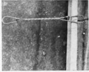
AB13035-BOOTH NO. 164-CONCRETE FORM TIES-Gates & Sons, Dept. AB, 80 S. Galapago St., Denver, Colo. Permitting easy assembly and dismantling of concrete forms, the one-piece combination tie and spreader is made of twisted wire with a loop at each end. Steel rods are dropped through the loops down each side of the concrete form, assuring foolproof fastening and perfect spreading. Ties are furnished in standard sizes from 6 to 60 inches: they may be used with any type of form-sheathing or nanel
