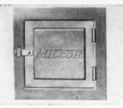
AB13064—CLEAN OUT DOOR—Inland Steel Products Co., Dept. AB, 4025 W. Burnham St., Milwaukee 1, Wis. The new door catch on the Milcor clean out door provides a positive locking action, preventing the door from being blown open. The new door hinge assures lasting freedom of operation, according to its manufacturer. The unit is stamped from 16-gauge copper alloy steel. It is furnished pointed. Size is 8 inches square. The clean out door is one of the many products in the Milcor building line.
