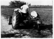
Power to lift and lower rear mounted tools. Line-Action hydraulic power from Ford Tractor's built-in hydraulic system gives you fast, sure control of rear mounted equipment.
