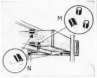
AB13082—ROLLER BEARINGS—Junior-Pro Products Co., Dept. AB, 3206 Morganford Rd., St. Louis 16, Mo. These devices are designed to prevent wooden drawers from sticking and binding, enabling them to be opened and closed with fingertip pressure, even in humid weather. Bearings consist of a plastic roller mounted on a steel pin and frame. Metal parts are cadmium plated to resist rust; each unit comes factory lubricated. Cement coated nails are furnished for an-the-spot installation.
