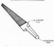
The handle end of a saw file makes a satisfactory substitute for an "Allen" wrench when cut to the size of the wrench desired.
