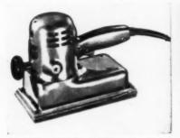
**AB13132—UTILITY SANDER**—The Black & Decker Mfg. Co., Dept. AB, Towson 4, Md. This sander produces 5,000 orbits per minute to give a satin-like finish; it will not track, score nor burn, and eliminates the need for final hand sanding. With a  $41/2x^{2}$  inch sanding surface, the bottom plate extends beyond the body of the tool for sanding close to obstructions. Switch handle is located close to the housing for better control, less fatigue.
