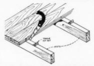
low space for the saw, the latter is inverted and a cut is made at an angle in the underside of the adjoining board on each side of the joist. The cut portion then is chiseled just below the upper surface of the board to free it from the nail.—Herbert E. Fey, New Braunfels, Texas
