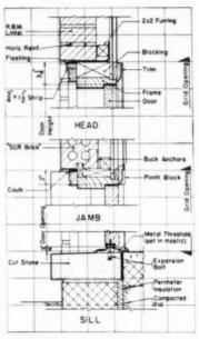
FIG. 2-Modular wood exterior door detail in "SCR brick" wall
