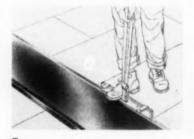
Flanges are bent upward to 90 degrees on the long edges of the initial strip —one-half inch high on one edge and one inch high on the opposite edge. Continuous strips up to 50 feet long can be used without cross seams
