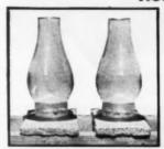
Prepare two slabs of mortar, one with Brixment and one with non-waterproofed materials. After mortars have hardened, seal a lamp chimney to each of the mortar slabs, using wax or candle grease, and fill with water.
