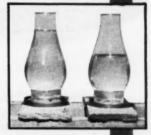
After 24 hours, note how much water has gone into and through the non-waterproofed mortar, and how little water has gone into or through the Brixment mortar.
