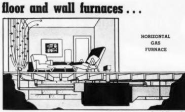
Horizontal gas furnaces offer economies in space, as they may be installed under basement ceilings, in utility room ceilings, or below the floor in crawl space for basementless homes. Locating the horizontal furnace in crawl space has also many duct-saving features, which also apply General Electric Data
