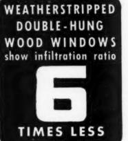
... than non-weatherstripped windows by actual test of weatherstrip manufactured by members of the Weatherstrip Research Institute. (University of Minnesota Institute of Technology Testing Laboratory.) Effectiveness is greater than 6 for average or poorly fitted windows.
