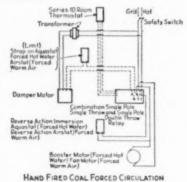
Hand-fired coal, forced circulation. This system has a thermostat, damper motor, transformer, limit control, and in addition, a relay to start and stop blower motor or booster pump motor. There is also a reverse-acting control in the voltage power circuit for starting the booster pump or fan motor in case the room thermostat is not calling for heat. This takes care of any
