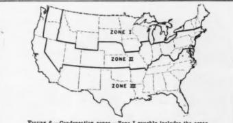
FIGURE 6.—Condensation zones.—Zone I roughly includes the areas with design temperatures  $-20^{\circ}$  F, and colder; sone, II 0° to  $-10^{\circ}$  F, and zone III areas warmer than 0° F.
