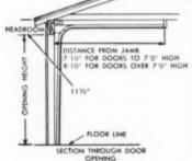
For good installation, lumber used in side jambs should be of good quality, straight, securely fastened to the structure, and not less than 15%" thick. Interior track support beam must be supported in center as well as at ends. With this, as with other garage doors, manufacturers furnish
