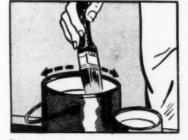
Dip it in about <sup>1</sup>/<sub>3</sub> the bristle-length. Tap gently on sides of can to "settle" the paint into the brush. Never scrape on rim of can. Always start with a clean brush.
