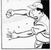
Joints, treated nailhead depressions and other surface irregularities should be lightly sanded to insure smooth receiving wall
