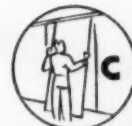
Doors are mounted in tracks by pushing doors into upper track, then engaging guide in floor guide.
