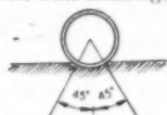
Bottom of pipe barrel, including 45° Arc from center, should be in firm contact with solid ground.
