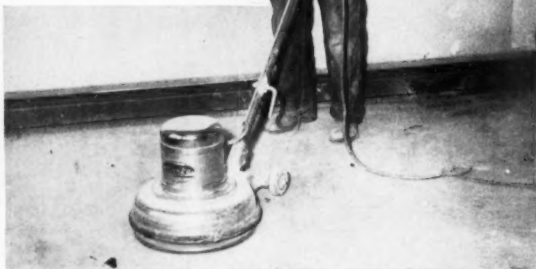
Slab sanding is the new way to clean the floor. Machine does the job in two hours
