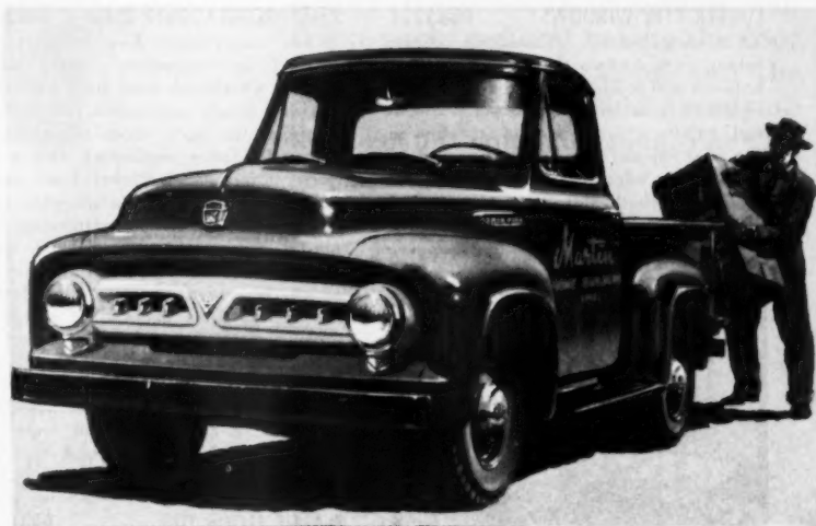
COMPLETELY NEW Ford Pickup with 6½-ft. box features new bolted construction, new clamp-tight tailgate. Choice of V-8 or Six. Five transmissions including FORDOMATIC DRIVE and OVERDRIVE (extra cost).
