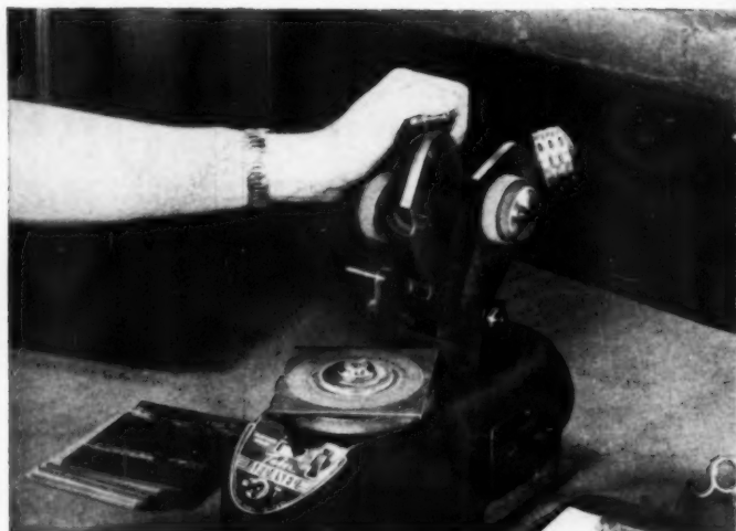
"The wear resistance of Kentile is controlled by frequent tests under the artificial 'foot' of this Taber Abraser."
