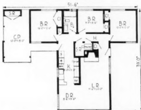
A good basic plan for project work on average-sized lots. Slab foundation. In Seattle, construction cost was just under $10.50 per square foot, on raw land
