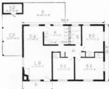
Furnace is located in hall, which has a 7-foot ceiling; other rooms have 8-foot ceilings. The one duct from the furnace connects with a ceiling diffuser in the living room. Outlets in hall heat other rooms
