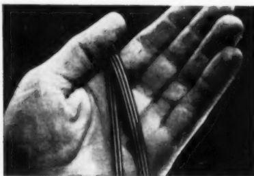
Small, lightweight wire used to connect switches with relays at fixtures or outlets.
