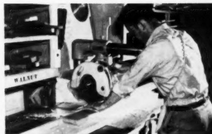
Sawing with saw table jig
