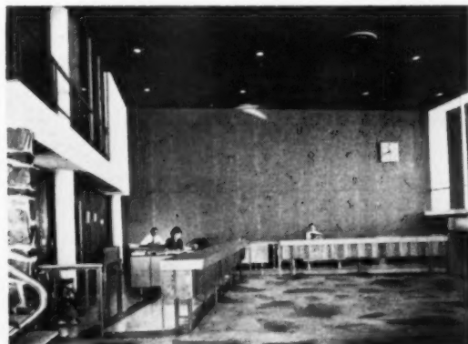
Traditional informality of the Southwest is reflected in the interior. Counters are of rough-sawn wood, floor is of native stone, and western brands are used decoratively on the wall
