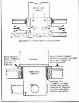
Two methods of plenum construction to assure safe operation
