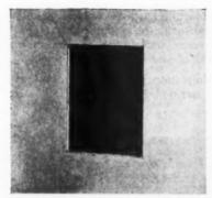
Cut-outs break clean. Trimming out for electrical outlets, etc., is easier, neater, because the Fiberglas reinforcements help keep the gypsum core from chipping off. Reinforced board is easy to score-and-snap or to saw.
