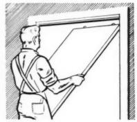
Hold rear door at angle and engage rollers on bottom of track. Let hang. Do same with front door. (30 seconds)
