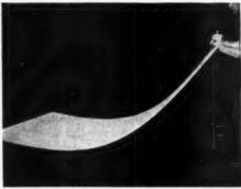
Improved flexibility. Fiberglas reinforcements help hold the board's gypsum core together, increase its flexural strength and resiliency. Means easier handling, greater resistance to cracking, chipping of edges and other damage.
