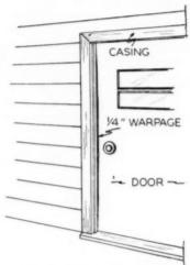
Warping is due primarily to differentials of moisture on the two sides of the door or differentials in temperature or both. Where these conditions are severe and the differentials are large, the likelihood of warping is always greater.
