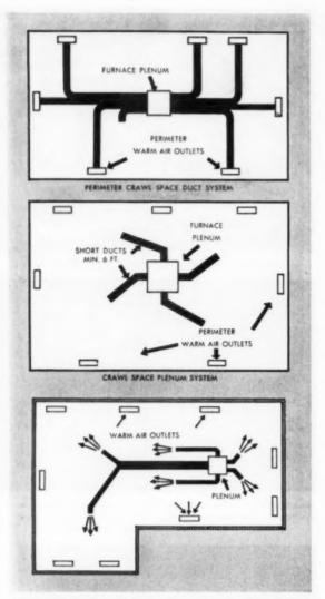
Three methods of crawl space heating: one using ducts to registers, the other two adapting the plenum system with stub ducts pointing to registers
