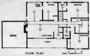
Floor plan showing position of ductwork in attic. Dimensions at diffusers refer to neck size as well as diameter of round duct. Sizes of all return ducts are noted under windows along exterior wall
