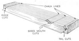
When cutting common rafters, make all ridge cuts first, using a power saw and an adjustable steel square or guide. Cut two rafters complete with bird's mouth cuts and tail cuts. Use these two completed rafters as patterns for cutting others.
