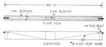
A 24-foot straightedge used to screed concrete must be without bow when suspended at each end, and should be light in weight. A straightedge that fits these requirements can be made in the following way: Two 1x6's that are 24 feet long are spaced apart with three 2x6 blocks (one placed at the center and one at each end). High test wire is used
