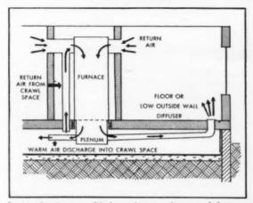
Section showing a modified crawl space plenum and duct system. Ducts provide warm air direct to registers and a duct provides warm air to plenum space
