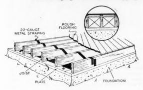
A simple and effective method of installing floor bridging is done with 22-gauge metal strapping about 11/2 inches wide. Strapping is laced in both directions and nailed to the top and bottom of each joist. This method of bridging of floor joists is much stronger than the average kind of wood bridging. Metal strap bridging does not tend to pull apart and it eliminates excessive cutting of lumber.-Bob Capps, Lombard, Ill.
