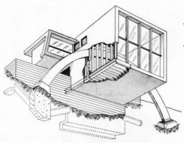
Footings supporting the arch are eight feet deep and are tied into the foundation. Anchor plates are secured to the piers by 18-inch bolts. Metal straps with turnbuckles for leveling hang from the arch and support the steel I-beams which form girders on which the projecting portion rests
