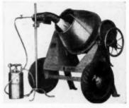
brackets. The "Fireblo" burner uses kerosene, distillate, diesel or light fuel oil and produces a quick, intense flame of over 2,000 degrees F. It is useful in thawing out concrete mixers, melting ice around foundations, pre-heating machinery. American Steel Works, Dept AB. 27th & Southwest Blyd., Kansas City 8, Mo.
