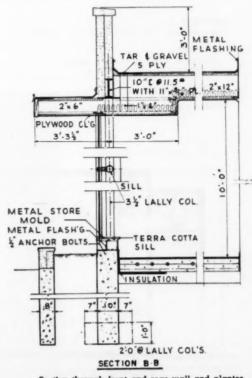
Section through front and rear wall and planter
