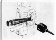
Boring jig clamped in its working position, showing hole saw guide in old lock hole
