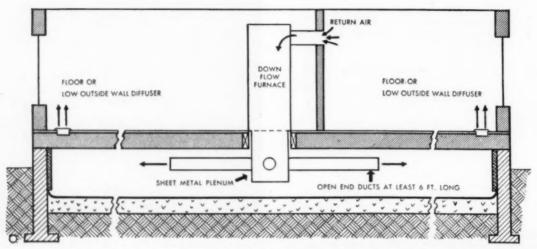
Sectional view indicating delivery of warm air into crawl space and from there into floor registers
