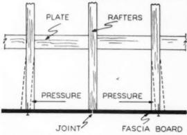
Sometimes fascia boards pull apart where they are joined, leaving an unsightly gap. To keep a fascia joint tight indefinitely, put pressure on the rafter tails away from the fascia joint as you nail each side of the two fascia boards. Then, when pressure is released, the relaxed rafter tails will force the fascia boards together into a tight-fitting joint.—C. E. Chubb, San Fernando, Calif.
