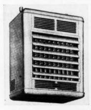
working zone and continuous circulation eliminates cold areas and stagnant air levels. Directional grilles permit the air flow to be controlled as desired. Threaded pipe hangers permit suspension of the heater in temporary locations, allow easy removal to other spots where needed, yet keep the unit up out of the working area. Four models are available, rated from 52,000 to 18,000 Btu's per hour. Utility Appliance Corp., Dept. AB, 4851 S, Alameda St., Los Angeles 58, Calif.
