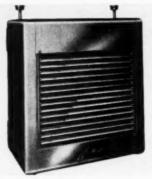
No piping systems or change-overs are required for temporary installations. Unit operates on natural, manufactured or LP gas. Heating capacities in nine models range from 50,000 to 225,000 Btu's per hour. Units are applicable to winter building, due to portability, capacities and minimum space requirements. Surface Combustion Corp., Dept. AB, 2375 Dorr St., Toledo I, Ohio.
