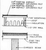
Here is a recommended built-up roof (with a 10 year bond) for a flat or slightly inclined deck showing joist and exposed beam construction. Quantities here are for 100 square feet.
