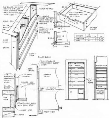
Upper left: details of closet liner, showing method of attaching %-inch boards to walls, fastening drawer supports; upper right: drawer construction details; lower left: filler block and hardwood support placement; lower right: front and side views with dimensions
