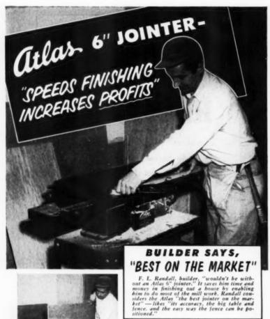
BIG CAPACITY Handling big boards is a sure, easy job on big Atlas working surfaces. THE TABLE IS 42" LONG! Fence, itself, is 32" long, 41/2" high. Fence quickly removes for surfacing wide boards.
