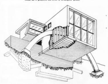
Footings supporting the arch are eight feet deep and are tied into the foundation. Anchor plates are secured to the piers by 16-inch bolts. Metal straps with turnbuckles for leveling hang from the arch and support the steel I-beams which form girders on which the projecting portion rests
