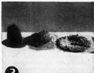
3 Design the mix for the job. These 3 (stiff, medium and wet) all are suitable, depending on where and how they are used.
