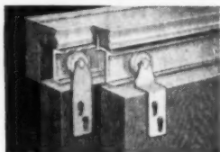
SCOTTIE SERIES Packaged kit—Low-priced hardware for \frac{3}{4} " to 1\frac{1}{8} " by-passing doors. Sturdy extruded aluminum track; taper-lock hangers with \frac{3}{8} " vertical adjustment.
