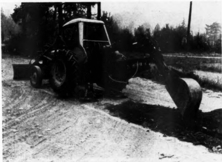
DITCHER: digs curb trenches, foundation footing trenches and secondary sewer and water-main trenches; also back fills with attached bulldozer blade
