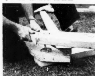
AB14262—SHERMAN—BOOTH NOS. 387-388—TRUSSED RAFTER —Timber Engineering Co., Dept. AB, 1319 Eighteenth St. N. W., Washington 6, D. C. Wood Frame Teco Trussed Rafter are fabricated on a special Teco designed rig. The rig is simple, lightweight and portable and can be built on the job by any carpenter without special tools or equipment. Precision assembly of trussed rafter joints is assured by use of the rig, Teco connectors, anchors and connectors (shown above) in conforming wedge-fit grooves.
