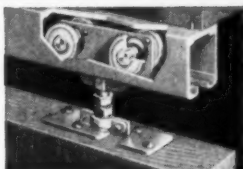
SERIES 400A Packaged kit—Also used in Series 800 KENNAFRAME... a prefabricated frame for pocket doors up to 150 lbs. Adjustable ball-bearing hangers; 8 wheels per door.
