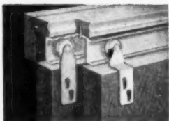
SCOTTIE SERIES Packaged kit—Low-priced hardware for \frac{3}{8} " to 1\frac{1}{8} " by-passing doors. Sturdy extruded aluminum track; taper-lock hangers with \frac{3}{8} " vertical adjustment.
