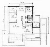
Plan contains 1.395 square feet of floor area and is laid out on a seven foot module. House can be turned in any direction and is designed so carport can be placed on any side (Continued on page 232)
