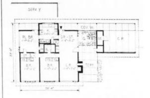
Plan contains 1,089 square feet of floor area. Rooms are centered around a "mechanical core, which serves both kitchen and baths. Lowered ceiling in bathroom makes the area above available for the installation of an air conditioning unit
