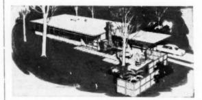
Roof slab is supported by columns independent of the exterior walls. This permits continuous window fenestration in the wall. The cantilevered roof slab makes possible wide overhangs
