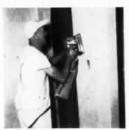
Now this new Model 127 Finishing Sander gets the dust before it gets you. Like a miniature vacuum cleaner, it sucks up the dust - traps it in a sealed bag. Keeps the room clean - the air clear.
