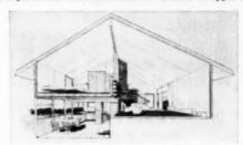
Section shows how living, sleeping and dining areas are separated, obtaining maximum usable floor space with split-level
