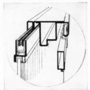
rolls on ball-bearing brass sheaves in the bottom rail on a stainless steel track.
