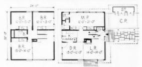
Plan contains a total of 1.582 square feet of floor area, which includes both levels. The house offers an abundance of living area with the formal portion at grade and recreation area one half flight down. Three bedrooms are located on upper level
