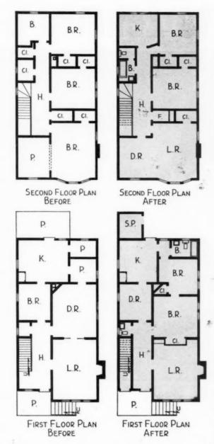
The before and after floor plan shows the use of the existing space. Few partition changes had to be made to provide the two 1,000-square-foot apartments
