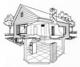
For air conditioning this 1600 square foot house, the Chrysler Airtemp air-cooled condensing unit is on outside. Operating cost for 1953 cooling season -\$48. In nearby house of similar area, water-cooled air conditioning cost \$72 to operate for same period. Inexpensive water rate held difference down in this case. Also, cost of maintenance of water-cooled unit was not considered!
