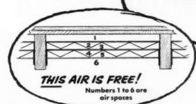
Multiple accordion aluminum as it comes compactly from package contains very little air:
