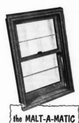
All MALT-A-MATIC Wood Window Units are fully weatherstripped and feature the "400" weatherstripping metals. Modular construction, plus the use of jamb liners, enables fitting in any thickness or type of wall.
