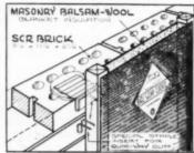
winter warmth. Masonry Balsam-Wool is vapor- and wind-resistant, bonded to the covering so it will not shake down in the walls. A flange permits it to be stapled or nailed to the furring strips. Wood Conversion Co., Dept. AB, First National Bank Bldg., St. Paul I, Minn.
