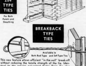
without reducing the tensile strength of the tie. Iden-tical to the regular galvanized Gates Form Tie plus Breakback feature. Leaves a hole only 9/64" in diameter that can be filled with any type wall finish. Break-back point occurs ¾" in from face of wall on Rod Type Tie and ¾" on 2x4 Type Tie.
