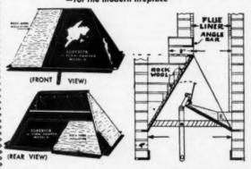
SUPERIOR HI-FORM Model "H" Damper is especially designed for modern fireplaces using a single smoke flue; such as a fireplace with the front and one or more sides open or, a fireplace opening through between two rooms (see section cut above). Superior Hi-Form is the only design damper we can conscientiously recommend for the modern fireplace.
