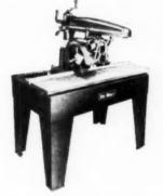
NEW MODEL GAO – 14" saw, 3 H. P., single phase. Cuts 4½" deep, rips to center of 48" panel. Used extensively for larger homes and industrial work where extra horsepower is needed. Standard arm model, only \$570, FO.B. factory. Other GA models available in 2 and 5 H. P.
