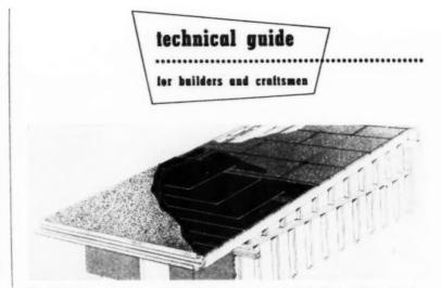
This illustration of built-up roof construction shows roof deck, built-up roofing, granules, gravel stop and gutter
