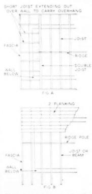
These short joists are anchored to a double joist over the main part of the house. This kind of structure is shown in Figure A.
