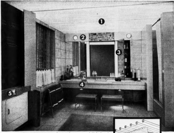
Rows of G-E Doluxo Warm fluorescent lamps are concealed behind panels of corrugated translucent plastic. Panels are lightweight, easy to install.
