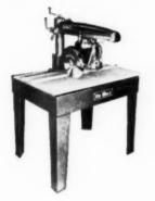
NEW MODEL GWH – 10" saw, 1 H. P., single phase. Built-in 110-220 volt change switch. cuts 3" deep, rips to center of 48" panel. Legs detach for portable use. Preferred by most small builders. Only \$395 delivered.
