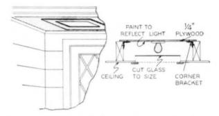
Recess a ceiling fixture at front or back door by cutting a square in soffit at desired spot. Frame opening with 1<sup>1</sup>/<sub>8</sub>-inch stock. Electrical fixture can be of a simple and inexpensive type. Cut glass to required size and insert through opening by tilting slightly. It is unnecessary to remove glass to change bulbs, Just shift glass to one side.
