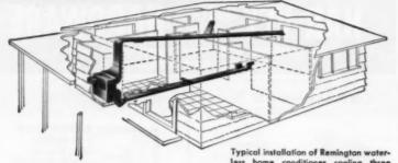
less home conditioner cooling three rooms. No water, piping, drains or water towers required. Heat and water towers required. Heat and moisture are exhausted outdoors.
