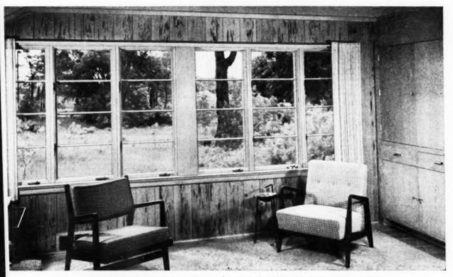
Andersen Casement Window. Beautiful Andersen Casements fit your plans perfectly. Available in many sizes, including picture window combinations. Choose from two sash widths (1' 6'' or 1' 10!/2''), five heights, one light, horizontal or cut-up glazing. Photograph shows paneled den featuring wide Andersen Casements.
