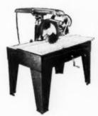
MODEL R-2K – Retractable arm. 12" Saw, 2 H. P., single phase. Built-in 110-220 volt change switch. Cuts 3½" deep, rips to center of 65" panel. Big 20" x 1" cut-off capacity – the finest value in the De Walt line at \$495 E O. B., Lancaster, Pa. This design has features that outmode all other makes. Also available in 3 and 5 H. P. 14" sizes.
