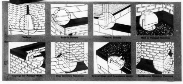
FOLLANSBEE SEAMLESS TERNE METAL, which is the original "Valley Tin," consists of copper-bearing steel strip coated with a lead-tin alloy. In addition to its use in valleys, Terne Metal is also widely used today for all types of flashings, for termite shields, for gutters and gravel stops, for copings and canopies, and anywhere else metal is used on all types of roofs, such as built-up, asphalt or asbestos shingle, tar-andgravel. slate, or tile.
