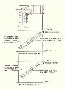
is tied on to the wall studs. The curve L-M is framed by short pieces L-N and O-M.
