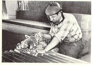
Corrugated or sheet aluminum is cut with metal slitting, mitre or cut-off blade. Mitre or cut-off blade is recommended for infrequent cutting. Use cutting oil or other lubricant. Lower foot to minimum depth of cut on thin sheets to achieve smoother cut
