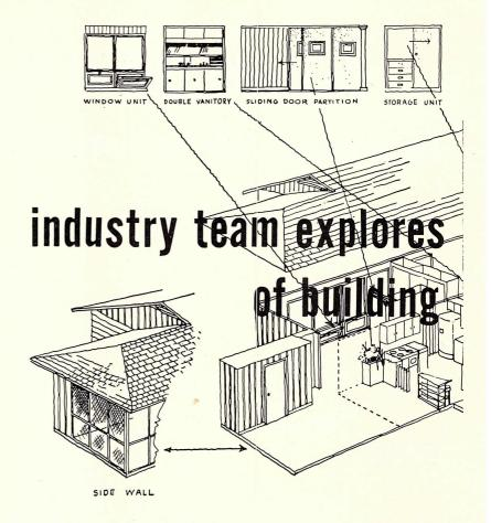
Fabrication or preassembly of as much of the house as possible, either on or off the site, has been the most dominant and persistent home construction trend in the postwar period.
