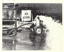
at the intake is not unusual, its makers say. It delivers its rated capacity when operating at the low speeds of 2,400 to 2,550 r.p.m.
