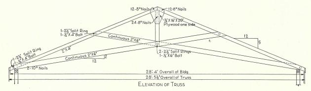
(I) Scissors truss can't take snow and dead-roof load of 35 pounds per square foot, a ceiling load of 10 pounds per square foot with spacing of trusses assumed at 24 inches on center. Below, typical living room showing interior studio effect achieved when scissors truss is used over living area
