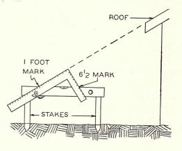
The pitch of any roof can be determined while you are on the ground if you use a common spirit level and a square. Drive two long stakes into the ground a suitable distance away from the building. Set the stakes about two feet apart. Be sure that the top ends are perfectly level.
