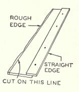
Uneven edges of boards can be quickly plumbed up without the use of a jointer by tacking on a straightedge to project beyond the edge of the board and parallel to the center line. Run the board through the table saw with the straightedge against the fence. This method is especially good for finishing S2S (surface two
