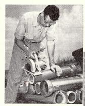
Clay tile pipe can be cut to size with little effort, using fiex cut-off wheel. Diamond grit is best for hard tile and fire brick
