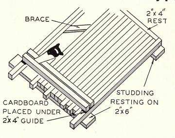
Use 2x4s and 2x6s to make this jig that will save you time when a great number of studs have to be cut. The length of the jig depends upon the length of the studs you plan to use. Its width should be such as to accommodate about a dozen studs at one time.
