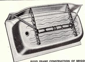
RIGID FRAME CONSTRUCTION OF BRIGGS TUB makes it free-standing! The framework is electrically welded to 24 spots on the tub—automatically fixes the tub in position, independent of wall support. Installation is much faster—considerably easier. Tub support and proper drainage are ensured.
