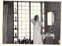
This attractive panel of Owens-Illinois Glass Block No. 365 allows in plenty of light, keeps out sight. An easy wipe keeps the panel bright and sparkling. A panel keeps the room warmer, too. Glass Block provide better insulation than a window and storm sash.
