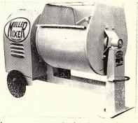
three-man crew. It is also useful to larger contractors as auxiliary equipment for use in places inaccessible to larger units. Weighing 195 pounds complete, it may be carried or hoisted to almost any location.
