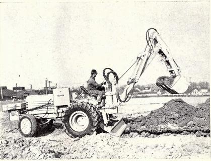
Bucket rotation of tractor attachment permits loading without spillage; boom has a full 200-degree swing. Stabilizer blade in front doubles as back-filler unit
