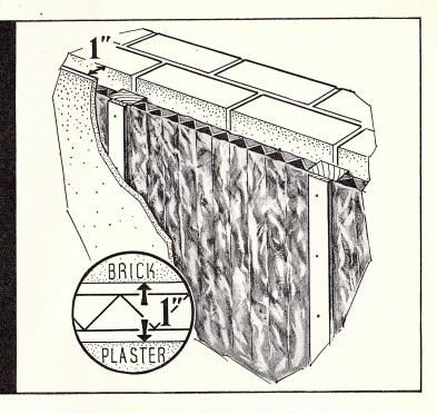
Masonry walls—brick, stone, cinder or concrete blocks—can be insulated against heat and vapor flow economically and effectively with 2 sheets of aluminum separated ½" apart by an accordion fiber. They can be attached in one operation to furring strips on the inside. Only ½" deep installed, they fit into the shallow 1" spaces created by the furring. The whole cost, material plus labor, should not exceed  $7\frac{1}{2}e$  sq. ft.
