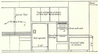
Counter top at right of oven built-in becomes a recess for a drop-leaf table built to fit underneath it and equipped with casters for easy use
