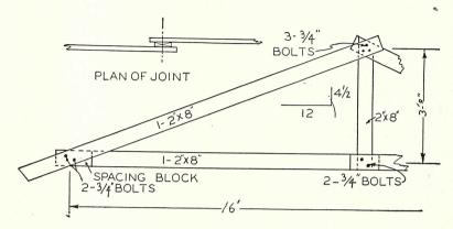
I am planning to build a home using wood trusses, with a shingled roof and either 1x8 V-joint boarding or plaster on the ceiling. I want to construct my trusses 16 feet in length at a 41/2 to 12 pitch with 30inch overhangs. I intend to space them two feet apart and use 2x6s for the rafter part, 2x4s for the joist part and a 1x6 for bracing. Is my thinking sound? How should the truss be designed?
