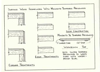
folks is the removable workbench top, which is made by fastening a piece of the Tempered Presdwood to a wood core with waterproof glue. This working surface may be used for sorting laundry and miscellaneous tasks, even including home workshop projects.
