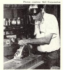
Steel can be cut with an abrasive flex wheel or a friction blade. Builder can use flex wheel on all material with good results. Use friction blade on steel up to 16 gauge and abrasive disc for heavier gauges or sections
