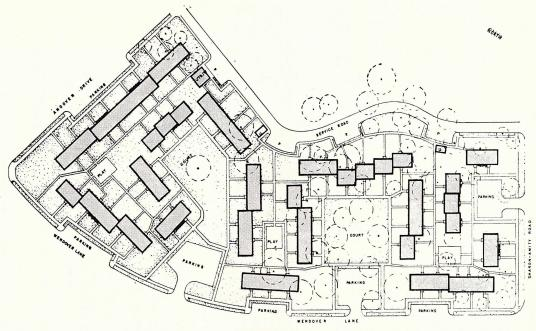
Typical block layout for rental housing. Each grouping of apartments has 1,200 square feet of playground, with slides, swings and teeter boards. Parking areas provide two car spaces per apartment unit
