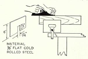
Cut two  $6x8\frac{1}{2}$ -inch pieces of  $\frac{1}{8}$ -inch cold-rolled steel. Then cut  $1\frac{1}{4}x3$ -inch notches so that they will fit over the threaded shaft and body of the vise. Put the plates in place and tighten the jaws of the vise.
