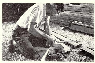
Flex wheel or cut-off wheel is used to cut metal pipe for perimeter radiator. Flex wheel is recommended for continuous cutting; cut-off wheel for occasional work
