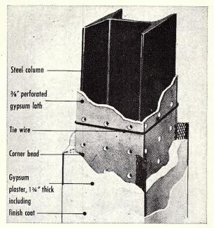
Perforated gypsum lath-lightweight aggregate gypsum plaster to provide three-hour fire resistance rating for steel column
