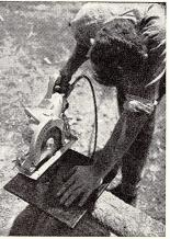
In cutting sheet steel, a friction blade is recommended on material up to 16 gauge. Abrasive flex wheel is best suited for heavier gauges or sections
