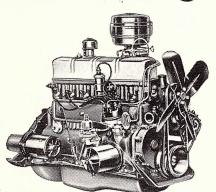
**New Low-Friction, High-Compression Cost Clipper Six** gives you more *usable* power from its 115 h.p. without boosting fuel costs. New Deep-Block design gives smoother operation, increases engine life.
