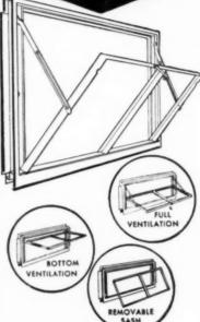
14-gauge electrically welded frame, fins welded to jamb for quick installation and double contact with leak-proof watershed sill. A plus value incorporates a redesigned latch which assures positive operation under all conditions.
