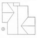
Figure A shows the solution to your roof problem including dimensions and the placement of hips and valleys at a 5 and 12 pitch. But with a maze of hips and valleys, it would seem to be expensive. You might consider a gabled-roof (figure B) which would be simpler to build and not as costly.
