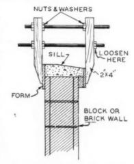
clamp quickly by loosening only the nut seen at the outside, right.
