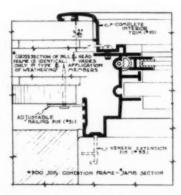
Cross section through the jamb shows the method of nailing the window to the building through the adjustable nailing fin. Distance between the interior trim and fin varies between  $4 \cdot 1/2$  and  $5 \cdot 5/32$  inches when fin is slipped into any of three channels
