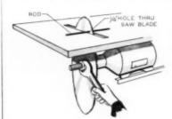
Drill a ¼-inch hole through the saw blade near the sawtooth edge. When you want to change blades, just slip a 12-inch length of ¼-inch drill rod about half way through the hole. The rod will hold the saw blade tightly and keep it from turning while you loosen the nut below to remove the blade.
