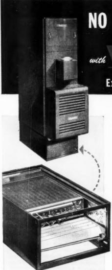
Illustrated above is the coil enclosure installed below a WILLIAMSON furnace. The evaporator coil is secured in a horizontal position. Below the coil are slanted fins which collect moisture removed in the air cooling process. A removable damper permits air to bypass the coil during winter furnace use. This unit is offered in a variety of sizes enabling it to fit most counterflow furnaces with belt driven blowers.
