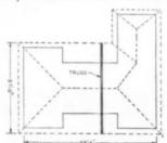
inches on centers across the portion of the house between the two porches with a 4-12 pitch strong enough to carry a plastered ceiling with radiant heating pipe panels imbedded in it. Roof is to be extra-heavy asphalt shingles over 30-pound building paper. How should this truss be designed?
