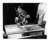
multi-purpose woodworking machine easily portable
