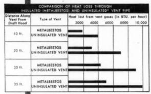
NOTE: Calculations based on 5" vent pipe with a height of 20' and a lateral run of 15'. Appliance input is 125,000 BTU. with 15,000 BTU. per hour assumed to reach the vent at the draft hond.
