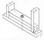
Header blocks can be placed between pairs of studs every eight feet along the foundation. Toenail studs to the sill and spike them to the ends of the headers with two 10d common nails, each side. Bolt headers securely to foundation.
