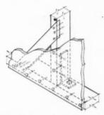
Sheathing, with 1x4-inch corner braces at 45-degree angle, from sill to plate, gives added rigidity. Nail sheathing with 11-gauge galvanized flathead roofing nails 134 inches long, 4 inches apart, 3x inches from edges and ends of boards.
