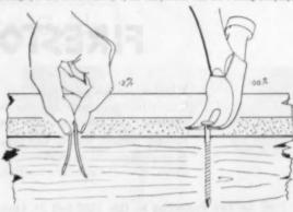
Driven into dry pine and withdrawn immediately, the average holding power of staples with divergent and V-points was 36 per cent of that of the threaded Stronghold nails. Six weeks after driving, the staple retained a 28-pound holding power as against 240-pound holding power for threaded Stronghold nail for the same period
