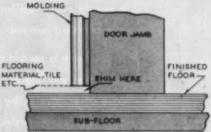
ing, simply put sample of floor covering on floor near door jamb, mark the thickness of the material on the molding and cut along this line. Then, when you lay the new floor surface, material will slide beneath molding easily.
