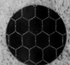
1. Keymesh woven wire galvanized reinforcing lath—applied over the gypsum or insulating lath on the entire ceiling, for highest quality, over all walls, lod. This network of multidirectional reinforcing increases strength, increases in safety 50%. Keymesh assures a uniform thickness of plaster, and guerds against cracks.
