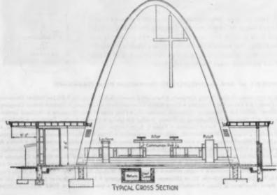
Cross section of church shows shape of basic parabolic arch, nine of which were used for interior spaced 12 feet on centers, Each arch spans a width of 34 feet, is 35 feet high. Aisles on both sides increase width of church to 45 feet
