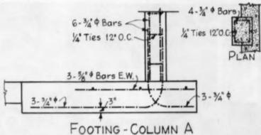
▲ Reinforced concrete columns support laminated arches. North and east walls are built of concrete block. West wall is of structural concrete. Curtain wall on east and north wall can later be removed should expansion of building become desirable ▼
