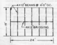
Place 4x12-inch beams 4 feet on center. Use number 1 clear, structural White Pine or Douglas Fir for the beams. Provide for a row of 4x12-inch bridging down the center, solidly cut in and spike well. Decking could be 2x6-inch T&G clear Fir with "v" joint. Provide a 2-inch rigid insulation and asphalt roofing if this roof is exposed to weather. No finish is required between beams on the decking inside, other than to sand, varnish and wax. Also sand, varnish and wax exposed beams.
