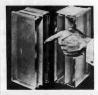
Glass blocks with diffusing screen to reduce glare
