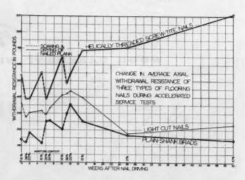
The chart indicates the change in average axial withdrawal resistance of three types of flooring nails during accelerated service tests
