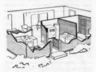
5. Grouping the kitchen, laundry, bath and the utility room or closet containing the air conditioner in one "core" saves installation cost. All of these require plumbing, gas lines or heavier electrical service
