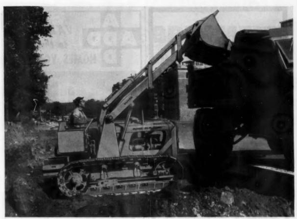
Oliver "OC-12" with hydraulic 1-yd. leader. This model has the long track frame for added stability. Loader has exceptional bucket rotation and 10' 4" leading height,
