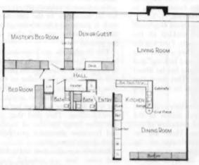
The shell of the house built with wall panels and roof trusses can be finished as one large room, thus making it possible to use non-bearing interior room dividers. The cost-saving techniques of this type of construction system are not limited in use to builders of large projects but have also been successfully adapted by the builder of few houses.
