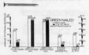
Average immediate and delayed withdrawal resistance of underlayment nails and staples driven through ¼-inch thick plywood or hardboard underlayment into dry or green southern pine
