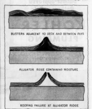
moisture. If it is applied during rain, snow or other types of damp weather, roof failure will result no matter how good the workmanship.
