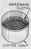
Make a dome-shaped insert from ½-inch square hardware cloth. Make the insert to fit a coffee can. With the insert in place in the bottom of the tin, the top of the dome should be about one inch from the bottom of the can. Add about two or three inches of your favorite liquid brush cleaner. The hardware cloth makes an excellent scraping surface for the brush, and the paint particles will settle to the bottom of the can. Brushes will be immersed in clear liquid cleaner at all times.
