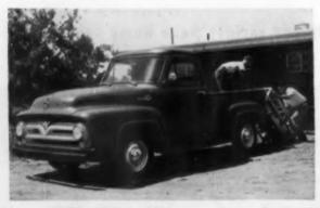
A new MONEY MAKER for light construction work—the '55 Ford F-100 Pickup with 5,000 lbs. GVW! Powered by the Short-Stroke 118-h.p. Cost Clipper Six or the Short-Stroke 132-h.p. Power King V-8, it carries top payload allowance . . . 1,718 lbs. Power Brakes and new Fordomatic Drive at extra cost.
