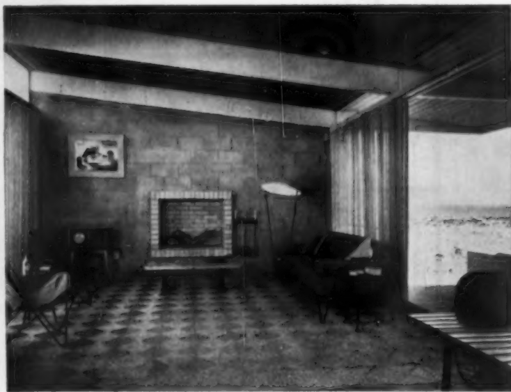
Living room and kitchen are left as one large room. Only separator is the eating bar, which makes possible an efficient U-shaped arrangement for kitchen cabinets and equipment. All ceilings have wood beams and 2 by 6-inch decking
