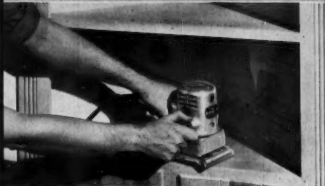
Black & Decker 88 Sander gives cabinets and other built-ins a perfectly smooth surface for final painting or staining.
