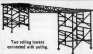
Two rolling towers connected with putlog.
