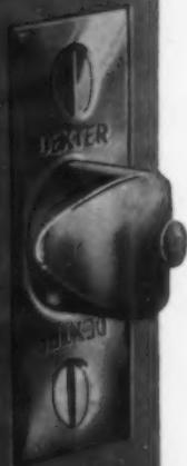
The Regal Line by Dexter includes this Colonial Design Tie Bolt Key-in-Knob Set with 6" dia. rose outside, 2 3/4" dia. rose inside and 5" backset. Available with pin or disc tumbler cylinder, deadlocking or spring latch. This new Dexter *Lifetime Lock* has solid brass exterior, cold-rolled steel interior parts. In standard or two-tone finishes.
