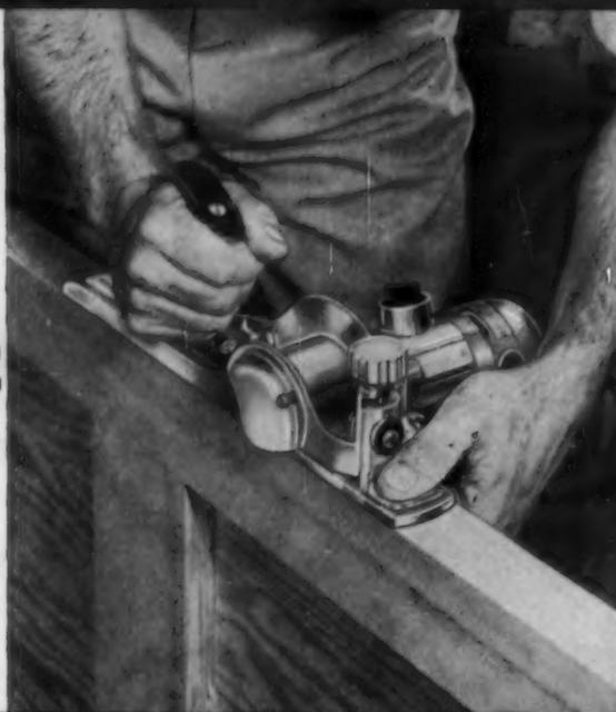
Here's a new Stanley jointer plane at a new low price. It's a big one, too; the shoe is a full 16" and the cutter width is  $2\frac{1}{16}$ ". The  $\frac{3}{4}$  hp, 20,000 rpm motor is interchangeable, can be used to power Stanley R8A Router and S80 Bench Shaper. Cuts
