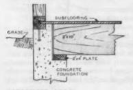
By providing a lip in the poured concrete foundation walls to accommodate 2x10 floor joists, it is possible to lower the floor approximately 8 inches. When the inside plates as well as the outside wall plates are placed, they are shimmed and gauged simultaneously for the width of a 2x10 floor joist.
