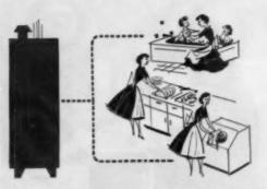
Washing clothes, dishes and the growing American family demands more gallons of hot water per hour, at varying temperatures. Appliances need about 160°, the optimum for 85% of the family wash; the skin takes about 110°. Builders should plan for potential need, with a 40-gallon tank and glass, rock or uncorroding metal linings as requirements. GAMA reports 1,393,500 heaters sold the first half of 1955, 23.3% over the first half of 1954, a trend aided by new shapes and compactness.
