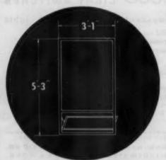
One of three basic sizes of Cace Fixed Windows with Nepper Ventilator used in Rolling Meadows homes. Two or three windows are joined with slender multions to achieve a picture window effect with adequate ventilation. Architect: A. J. Del Bianco, Chicago, III. Carpenter Contractor: Joseph T. Carp, Inc., Chicago, III.
