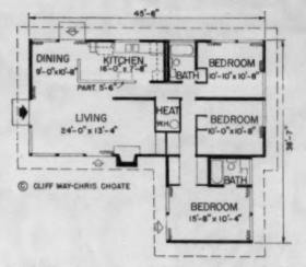
**PLAN** shows four entrances, which contribute to flexible placement on lot. Heating unit at center connects by ducts in slab to perimeter diffusers. Gas is natural in Texas, the largest supplier. Sleeping quarters form separate wing.
