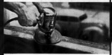
New Black & Decker 7-inch Sander-Polisher makes short work of paint removal; provides better surface for re-painting.
