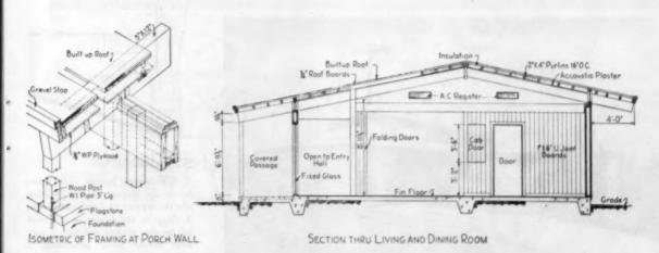
Inside-outside harmony is strengthened by use of vertical 1x6 V-joint boards, finished with driftwood stain, both for siding and paneling
