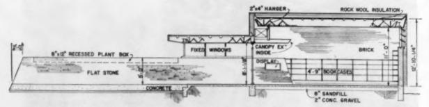
LONG AND LOW entrance wall of erab orchard stone leads past door into reading room, has built-in plant box. Ceiling has 4-inch rock wool insulation. Duct above canopy contains air conditioning vents. Canopy hangars are 2 x 4's.
