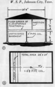
In your problem, a 3-inch nominal diameter pipe column (actual dimensions are 3.5 inches outside and 3.068 inches inside) can carry 30,000 pounds on an unbraced height of 8 feet, and 26,000 pounds on an unbraced height of 10 feet. The allowable load decreases as the laterally unsupported height increases, because of the additional danger of buckling.
