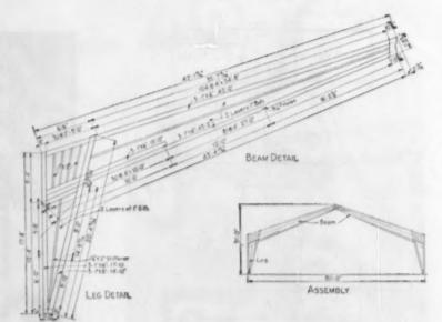
other job, beams exceeding 350 feet in length were practical because beams were delivered in lengths of approximately 80 feet and then joined on the site.
